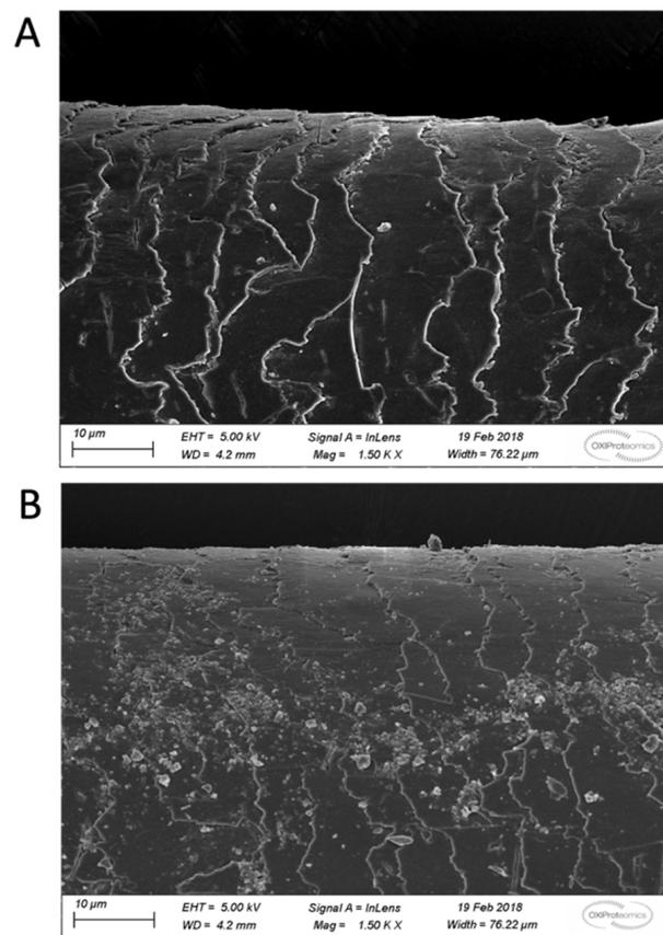
**Figure 2.** The adhesion of particulate matters on hair surface is detected and presented by image collection via scanning electron microscopy (SEM). (A) Not treated hair fiber; (B) hair fiber exposed to airborne pollutants (PM).
