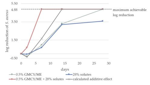
**Figure 4.** Plot of the log reductions in *S. aureus* in the o/w emulsion containing either 28% solutes, 0.5% Glyceryl Caprylate/Magnolia Officinalis Bark Extract or both systems in combination as well as the calculated additive effect, which results from the addition of the individual systems. The maximum achievable log reduction was 4.88;, therefore, the additive effect (if it exceeded this value) was set to 4.88.
