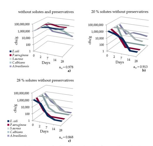
**Figure 2.** Challenge test results of the o/w emulsion (**a**) reference without solutes ( $a_w = 0.978$ ), (**b**) with 20% solutes ( $a_w = 0.913$ ) and (**c**) with 28% solutes ( $a_w = 0.868$ ), indicating the colony-forming units (cfu/g) for the germs *E. coli*, *P. aeruginosa*, *S. aureus*, *C. albicans* and *A. brasiliensis* after 2, 7, 14 and 28 days.
