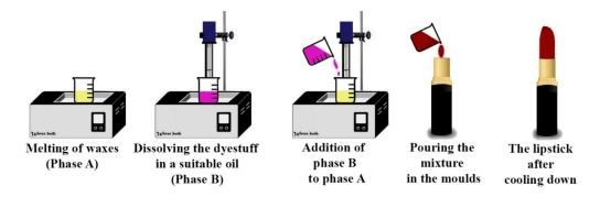
Figure 1. The general method of preparation for lipsticks.
