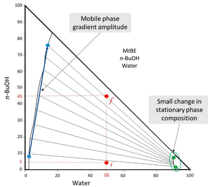
**Figure 2.** Ternary diagram of MtBE/*n*-BuOH/water: type 2 diagram allowing a fractionation by gradient elution CPC. Red markers refer to initial (i) and final (f) conditions. Green and blue markers refer to the composition of lower and upper phases, respectively. Compositions in terms of MtBE/*n*-BuOH/water for initial mobile phase 89/8.5/2.5 (v/v/v), final mobile phase 7/76/17 (v/v/v), initial stationary phase 7.5/1.5/91 (v/v/v) and final stationary phase 7/3/90 (v/v/v).
