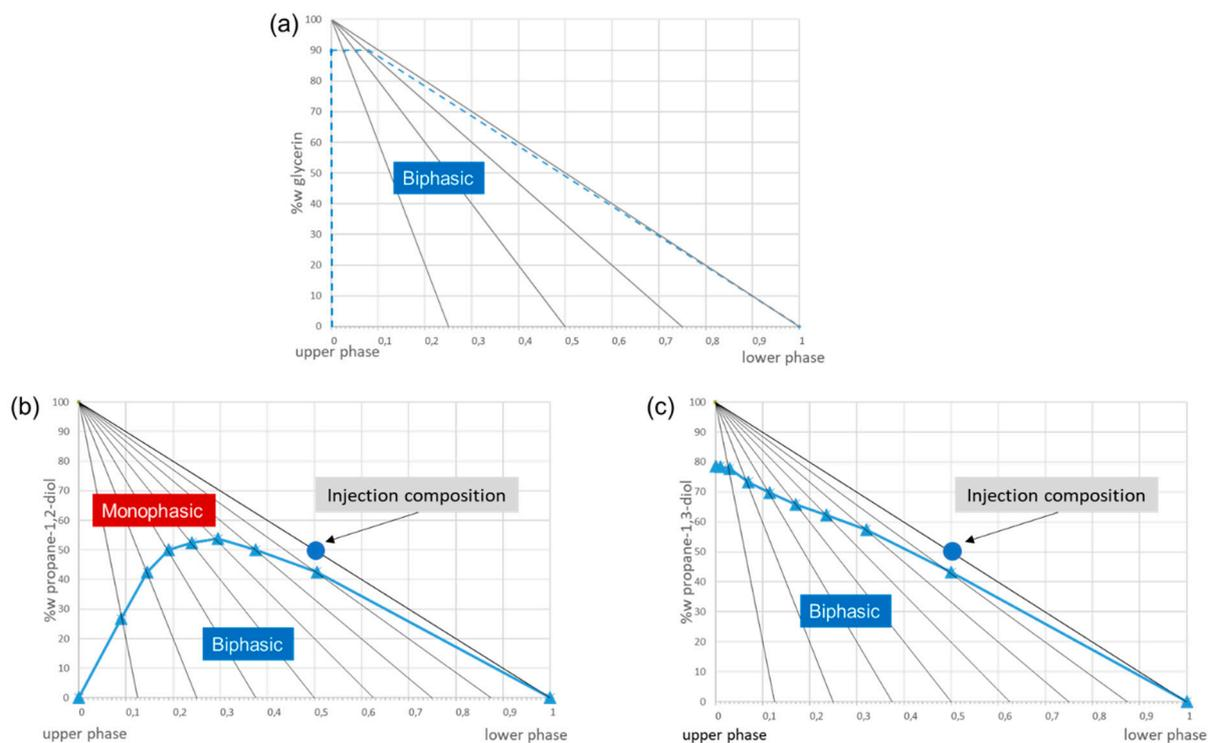
**Figure 3.** Ternary diagram of upper phase, lower phase and (a) glycerin, (b) propylene glycol and (c) propanediol for the MtBE/*n*-BuOH/water 45:5:50 (v/v/v) solvent system. Demixing points are symbolized by triangles in (b,c), while in (a), none were observed before the addition of 90% by weight of glycerin (maximum points studied).
