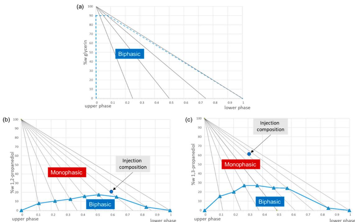
**Figure 1.** Ternary phase diagram of upper phase, lower phase and (a) glycerin, (b) propylene glycol, (c) propanediol (*w/w/w*) for the EtOAc/CH<sub>3</sub>CN/water 3:3:4 (*v/v/v*) solvents system.
