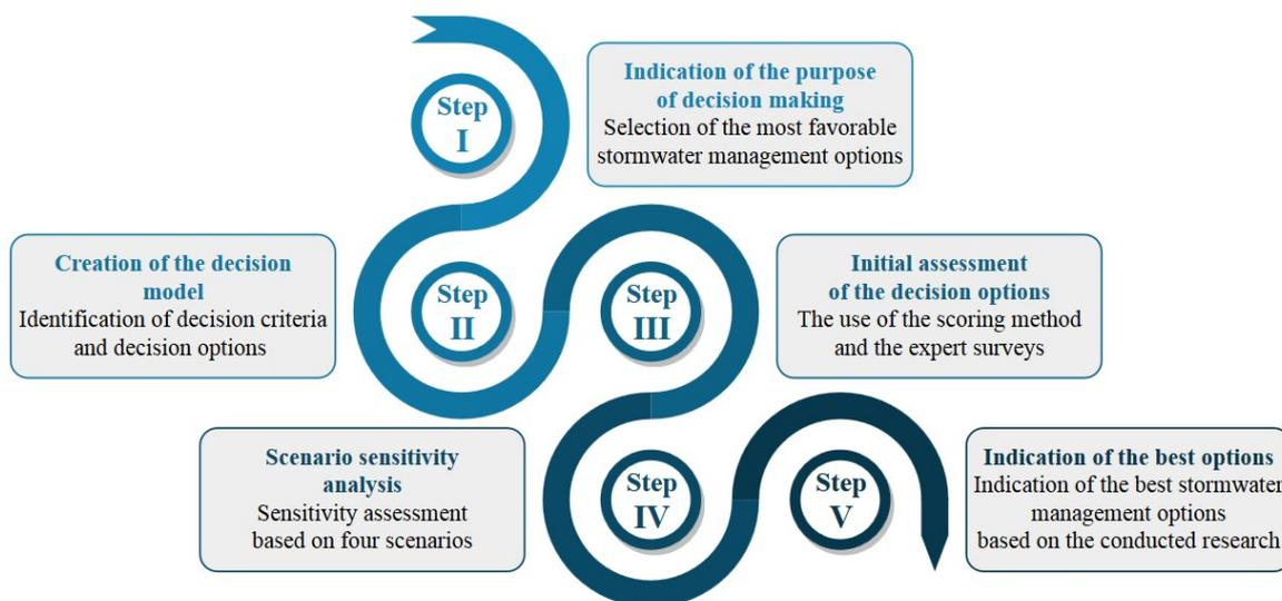
**Figure 1.** The procedure for selecting the most advantageous method of stormwater management discharged from the area of newly designed multi-family housing estates.
