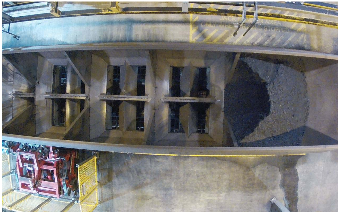
Figure 1. Coal hang-up in front compartment of wagon.
