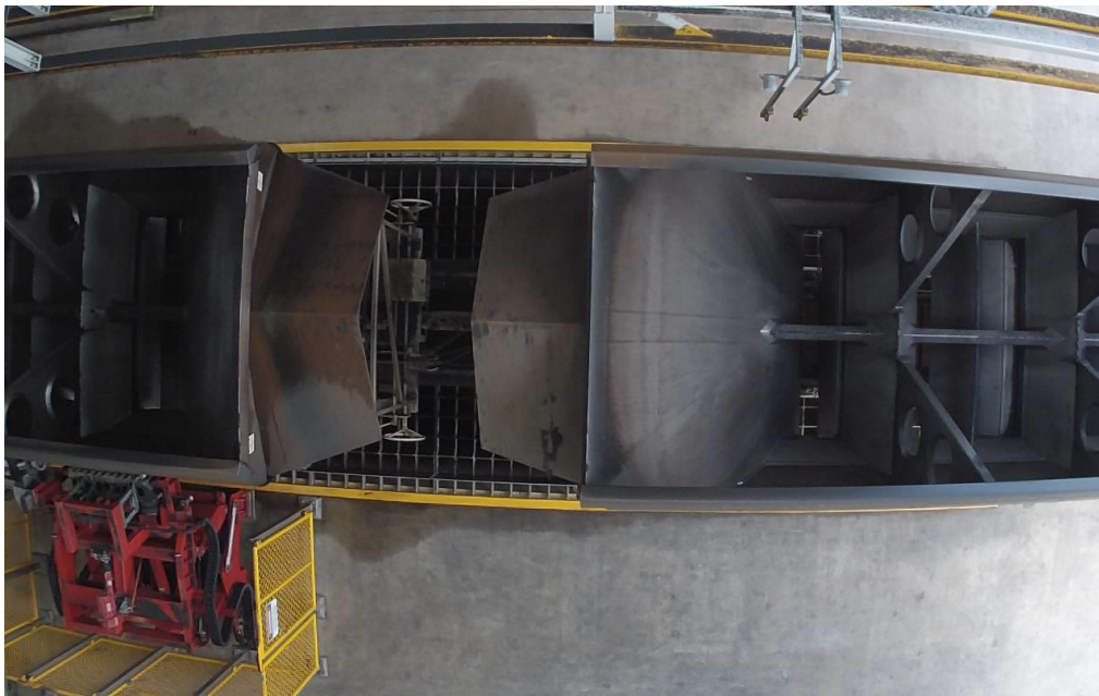
Figure 10. False alarm triggered by wagon paused directly under the laser scanner.
