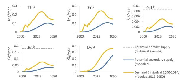
FIGURE S3: THE DEMANDS BY AEV INFLOWS AND POTENTIAL SECONDARY SUPPLIES FROM END-OF-LIFE AEV OUTFLOWS OF THE RARE EARTH ELEMENTS TB, ER, GD, PR, AND DY IN THE USA, 2000-2050, AND HISTORICAL (2012-2015) AVERAGE DOMESTIC PRIMARY PRODUCTION (GD AND PR ONLY) SUPERIMPOSED. NOTE THE DIFFERENT ORDINAL SCALES.
