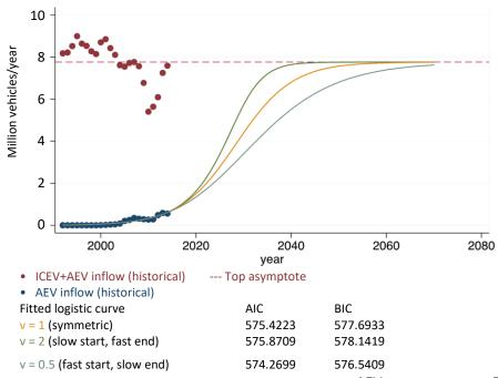
FIGURE S2: COMPARISON OF THREE LOGISTIC CURVES FITTED TO THE HISTORICAL AEV INFLOW DATA AND 7.76x10<sup>6</sup> TOP ASYMPTOTE, WITH DIFFERENT VALUES OF V. ALSO SHOWN ARE THE AIC AND BIC STATISTICS OF THE THREE FITTED CURVES.
