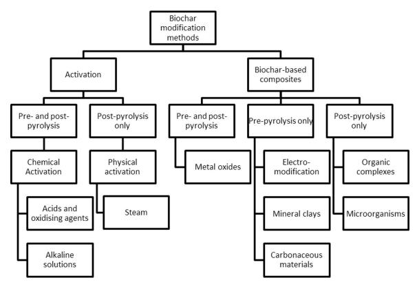
**Figure 2.** Biochar modification methods to enhance properties. (Reprinted from [121], with permission from Elsevier). © 2017 Elsevier Ltd.
