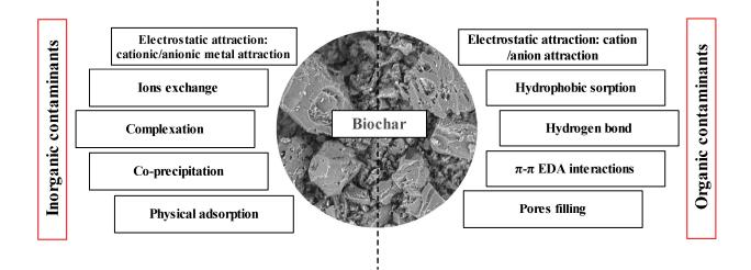
**Figure 6.** Mechanism of pollutant removal from water using granular carbonaceous materials (Reprinted from [221]). © 2020 by the authors.
