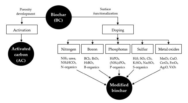
**Figure 4.** Elements and compounds used to improve the biochar structure. (Reprinted from [120]). © 2018 by the authors.
