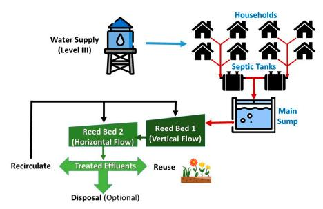
**Figure 3.** Flowchart of a wastewater treatment system using constructed wetlands in the City of Bayawan, Negros Oriental.
