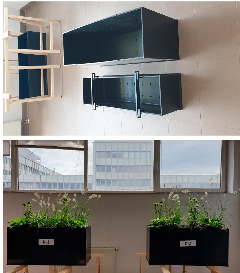
**Figure 4.** Bioretention drainage channel modules installed in the laboratory.
