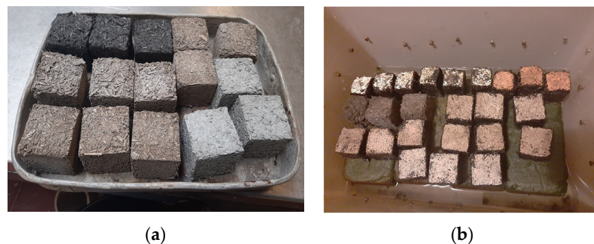
Figure 6. (a) prepared samples; (b) capillary absorption test (samples on water saturated oasis).
