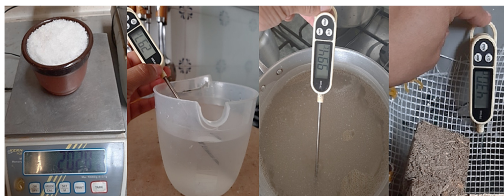
Figure 9. Temperature-controlled salt vapor preparation process.
