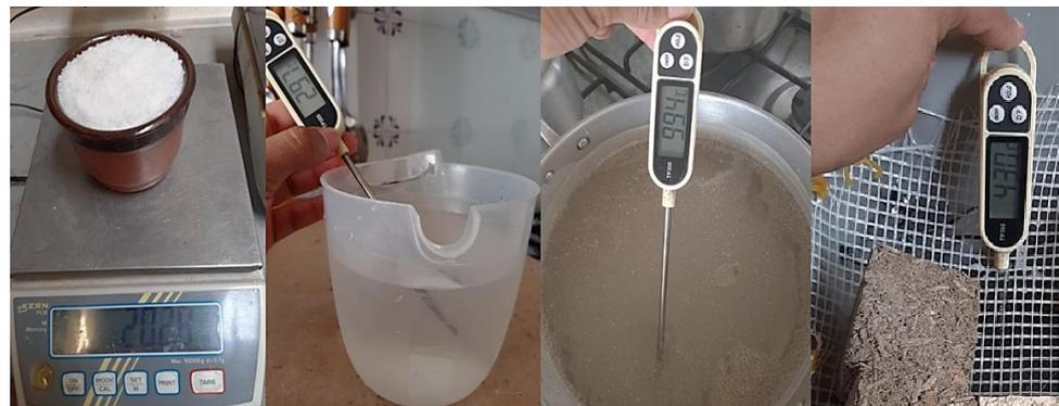
Figure 9. Temperature-controlled salt vapor preparation process.
