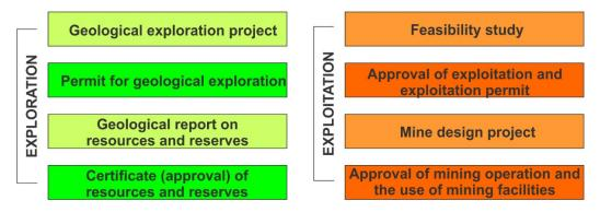
**Figure 2.** General procedure for permitting in Serbia with all necessary documents (light colour) and corresponding certificate/approval/permit (darker colour) for the whole mining cycle. Other important documents at certain stages are discussed in the text.
