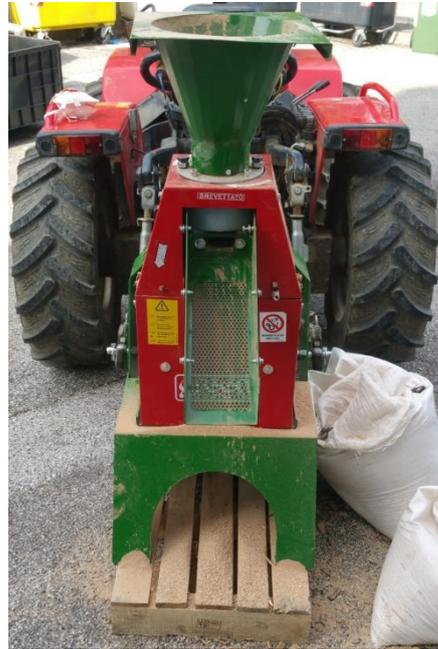
**Figure 1.** Green Technik mod. PTM50, pelletizer used for the production of pellet samples in the small-scale company.
