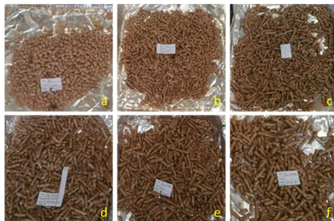
**Figure 2.** (a–f) Pelletizer regulation tests: pellet results produced with a decreasing distance between rollers and die from test (a) to test (f).
