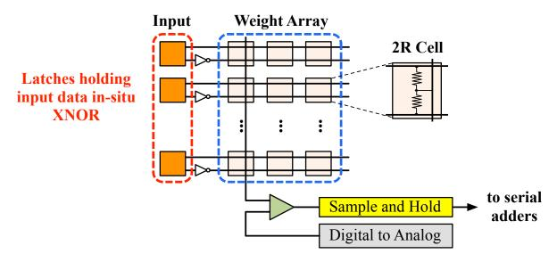
Figure 12. In-situ XNOR operations within the proposed memory array.
