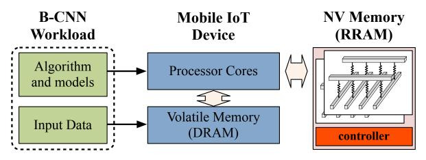
**Figure 6.** Accelerating B-CNN workloads with the proposed memristive binary convolutional architecture. The RRAM crosspoint arrays are used for storing data and performing in-situ XNOR convolution.
