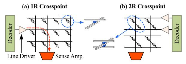
Figure 5. Illustrative examples of 1R (a) and 2R (b) crosspoint arrays.
