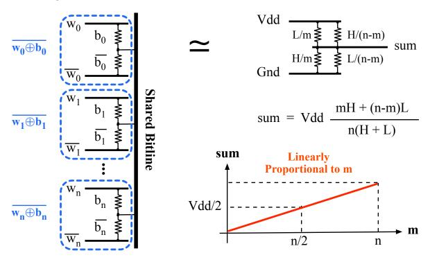
Figure 8. Performing bit-count operation within the 2R crosspoint array.
