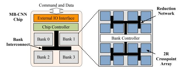
Figure 10. The proposed hierarchical organization for the accelerator.
