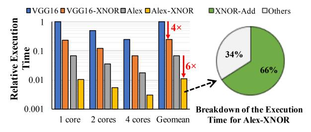
Figure 1. Impact of XNOR convolution in state-of-the-art neural networks.
