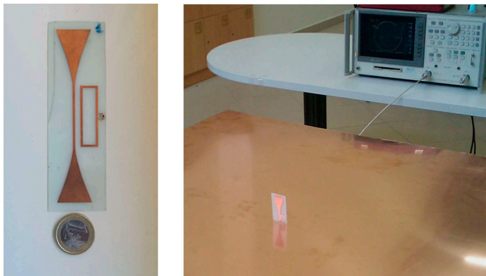
Figure 8. Antenna prototype (left) and antenna input impedance measurement set-up (right).
