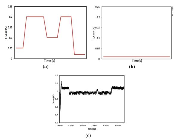
**Figure 11.** Current traces generated from running benchmark and including them in Cadence ADE as load. (a) upper stack load; (b) lower stacked loads; (c) 2:1 Down converted Vout  $(Vdd = 2 V, Vout \sim 1 V)$ .
