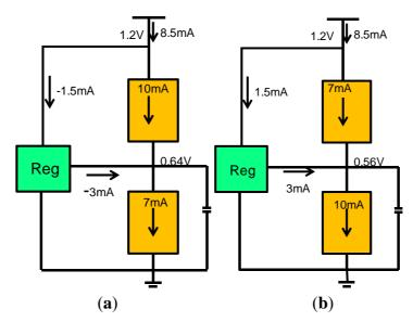
Figure 3. (a) Illustrates the push-pull switched capacitor designed to assist voltage stacking;
