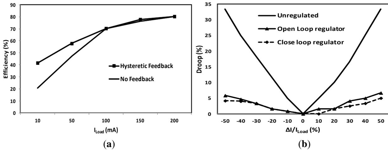
As Figure 8a shows, the feedback circuit has considerable impact on efficiency for conventional load, especially at lower current. However stacked load has unique characteristics which are explained below with the help of Figure 1a [9].
