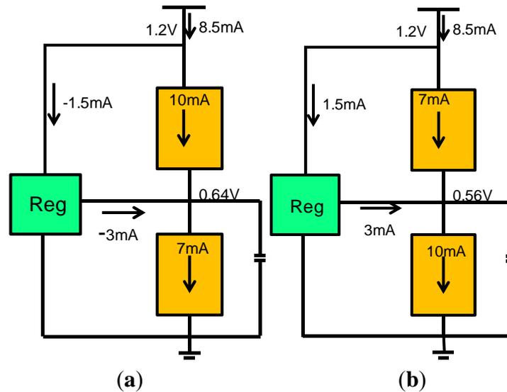
**Figure 3.** (a) Illustrates the push-pull switched capacitor designed to assist voltage stacking; (b) Fly-capacitors are swapped over the phases to regulate the *imbalance* between the stacks. Arrows indicates the direction from which charges are flowing to and from  $V_{out}$ .
