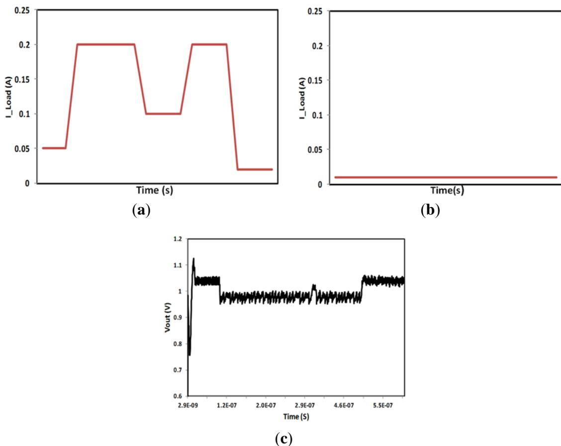
**Figure 11.** Current traces generated from running benchmark and including them in Cadence ADE as load. **(a)** upper stack load; **(b)** lower stacked loads; **(c)** 2:1 Down converted Vout (Vdd = 2 V, Vout ~ 1 V).
