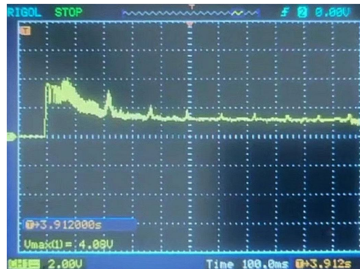
Figure 9. Starting current diagram of actual motor operation.
