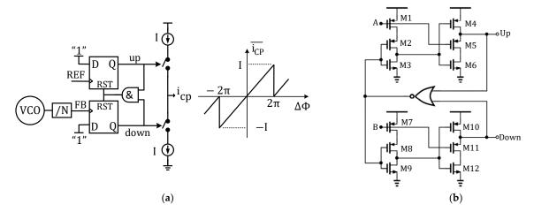
**Figure 1.** (a) Structure of a conventional three-state PFD and CP and its linear transfer characteristic; (b) TSPC PFD structure.
