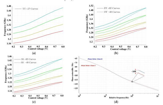
**Figure 11.** Simulated VCO tuning curves (a) typical (TT), 27 °C; (b) fast (FF), 85 °C and FF, -40 °C; and (c) slow (SS), 85 °C and SS, -40 °C; (d) VCO simulated phase noise showing both class-B and class-C performance.
