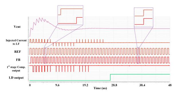
Figure 9. Simulated performance of the proposed lock detector.
