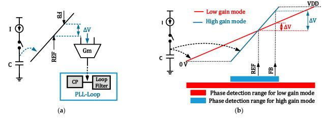
**Figure 3.** (a) Conceptual structure of the proposed LSPD (translating phase error into a voltage difference and then converting it into current injected into the loop filter); (b) trade-off between phase detection gain and range.
