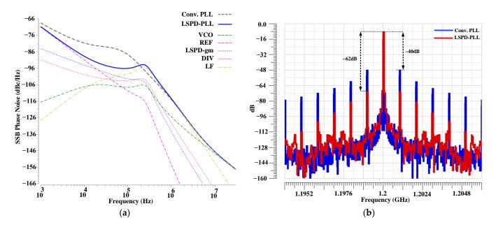
**Figure 13.** (a) Simulated phase noise performance of the proposed INPLL compared with that of an INPLL that uses conventional PFD-CP; (b) simulated output spectrum of the proposed INPLL compared with that of an INPLL that uses conventional PFD-CP.
