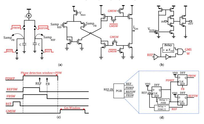
**Figure 4.** (a) Schematic of the proposed LSPD-Gm; (b) tunable delay cell and GMSW pulse generation circuit; (c) timing diagram of LSPD pulses; (d) Pulse Generator Block (PGB); (REF-IN: Input Reference, PDWP: Phase Detection Window Pulse, REF: input to the loop, GMSW:  $G_m$  window pulse, REFSW&FBSW: pulses determining the charging interval of the sampling capacitors).
