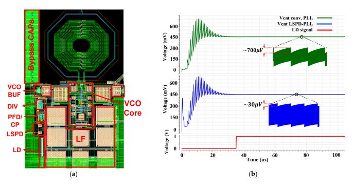
**Figure 12.** (a) The layout view of the proposed INPLL; (b) simulated settling behavior of the proposed INPLL compared with that of an INPLL that uses conventional PFD-CP.
