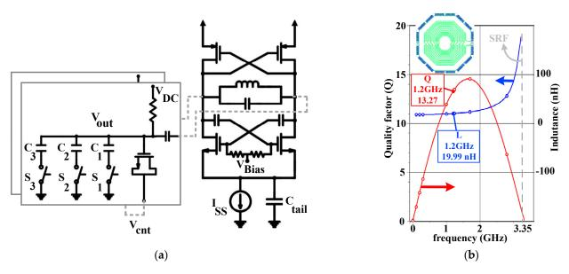
**Figure 10.** (a) Class-C LC VCO Schematic; (b) simulated performance of the designed inductor (SRF: Self-Resonance Frequency).
