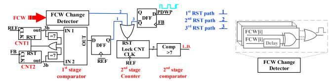
**Figure 8.** Block diagram of the LD showing both stages and the reset paths (FCW: Frequency Control Word).
