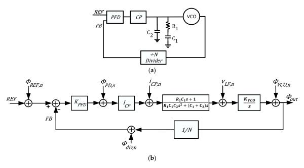
**Figure 2.** (a) Architecture of the conventional INPLL; (b) linear phase domain model of conventional PFD-CP PLL.
