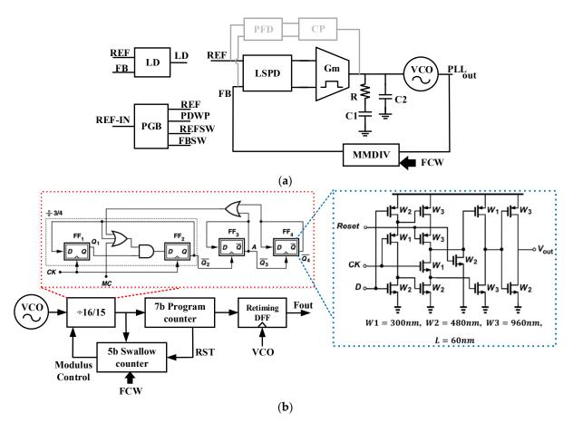
**Figure 6.** (a) Block diagram of the proposed INPLL (details of PGB and LD are explained in Figure 4d and LD's section respectively); (b) utilized MMD structure.
