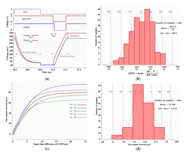
**Figure 5.** Simulated performance of the proposed LSPD showing: (a) transient response during the phase detection; (b) Monte Carlo results of the phase detection gain; (c) Gm output current across process corners and temperature; (d) Monte Carlo results of the Gm output current for various input timing errors.
