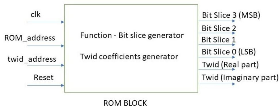
**Figure 10.** Black box representing the ROM BLOCK with the relevant input and output signals.
