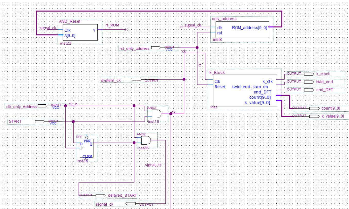
**Figure 8.** Schematic design of the timing block.
