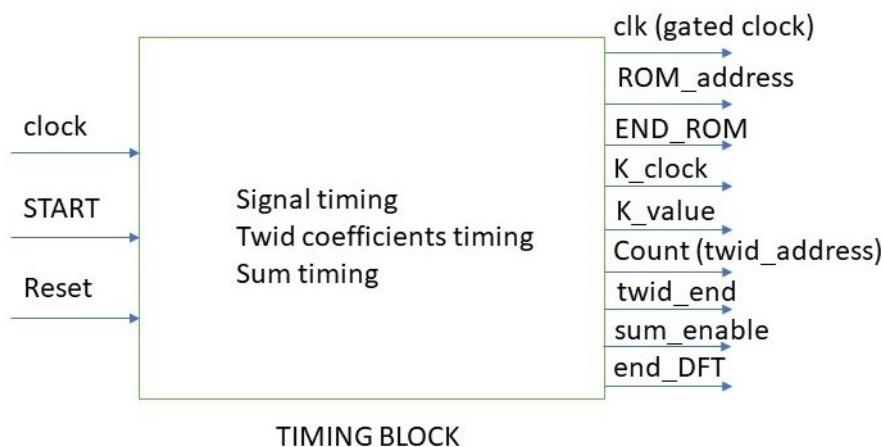
**Figure 7.** Black box representing the timing block with the relevant input and output signals.
