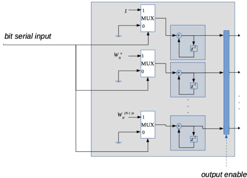
**Figure 4.** Logical scheme of a generic BFT block having samples of a bit slice as serial inputs.
