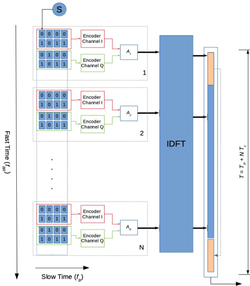
**Figure 5.** The 16-QAM OFDM modulation scheme.
