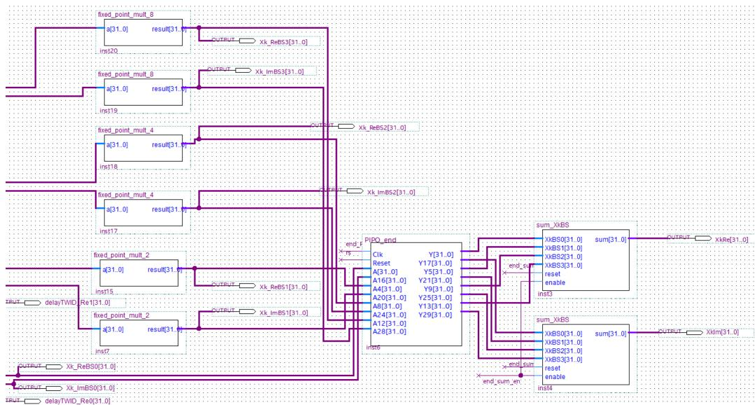
**Figure 15.** Schematic design of end\_sumBlock.
