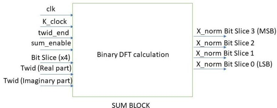
**Figure 11.** Black box representing the SUM BLOCK with the relevant input and output signals.
