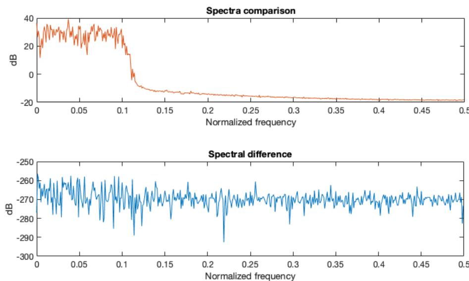
**Figure 18.** Spectra comparison between Matlab double precision FFT and the proposed approach.
