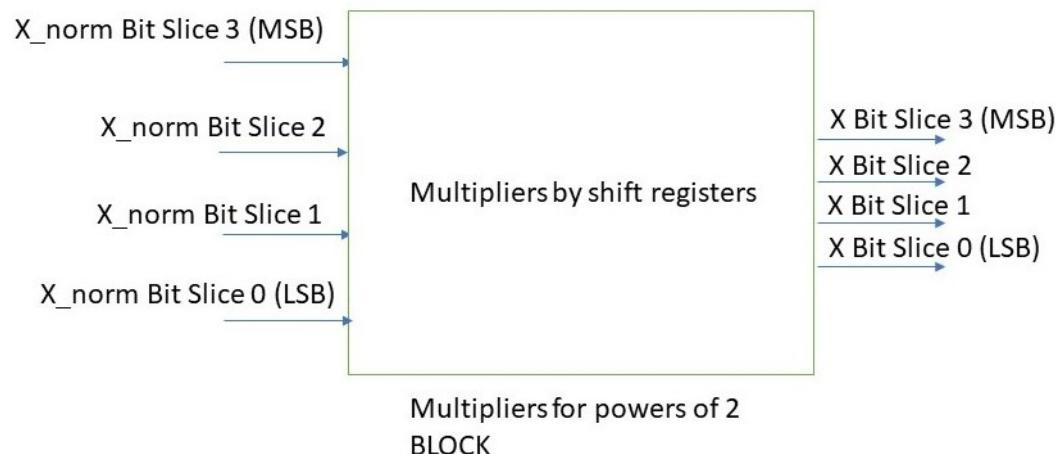
**Figure 16.** Black box of the multiplier module with input and output signals.
