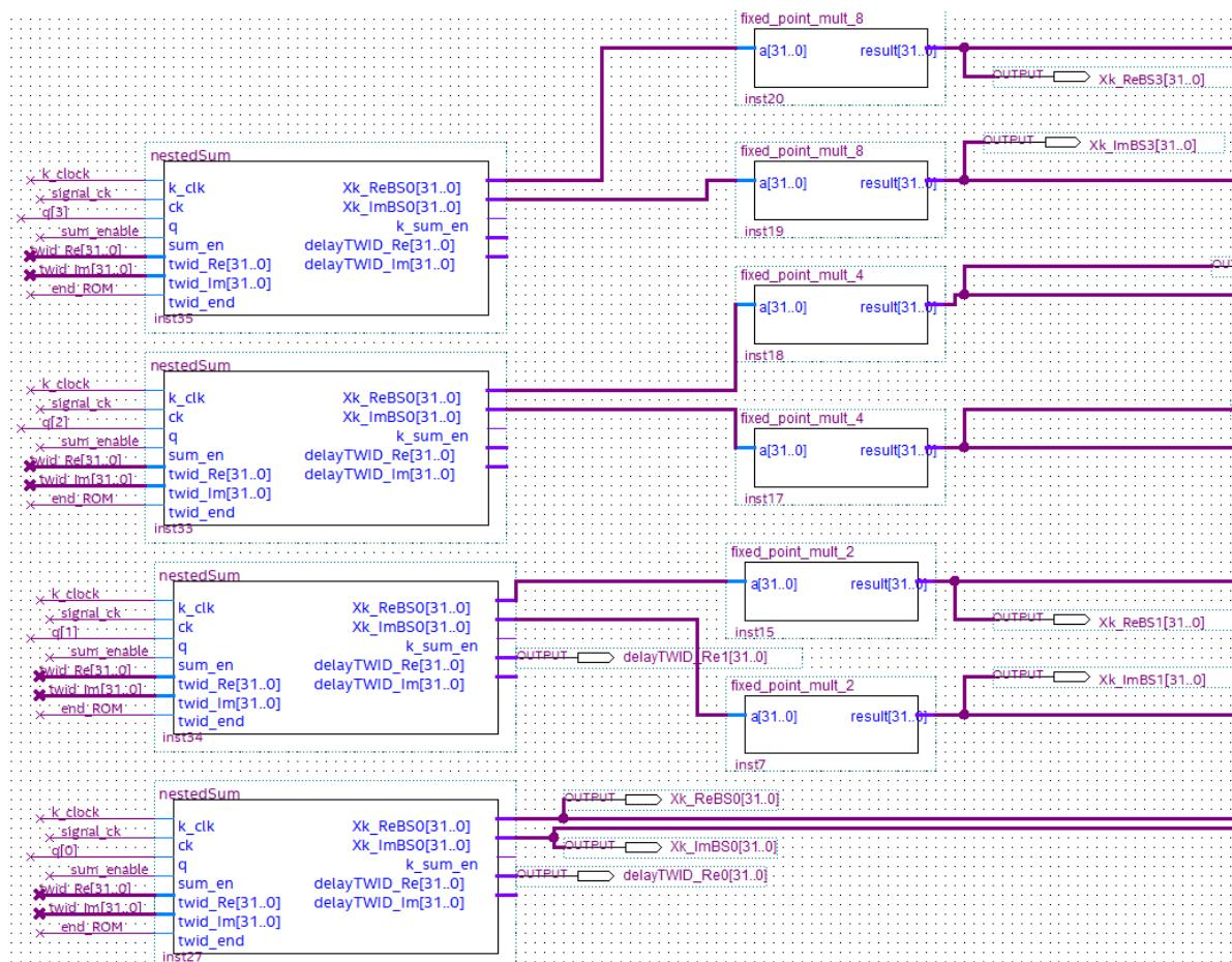
**Figure 12.** SUM BLOCK schematic.
