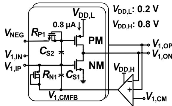
Figure 3. Schematic of SQI  $C_{S1} = 1$  pF,  $C_{S2} = 4$  pF.
