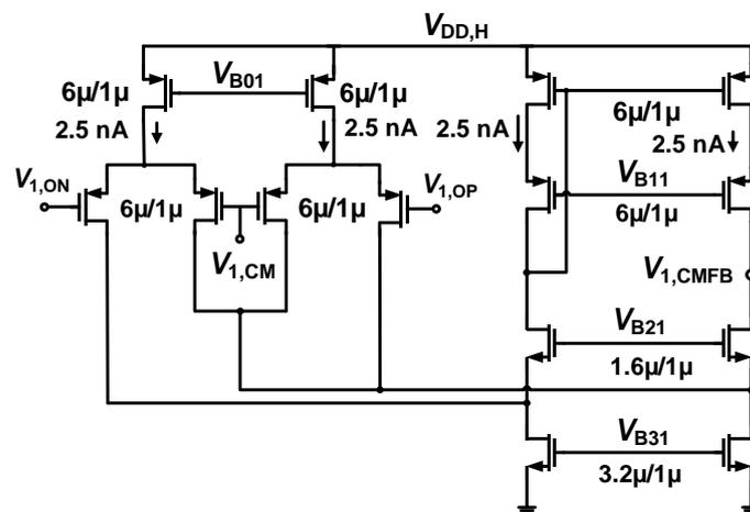
Figure 4. Schematic of CMFB circuit of the SQI.
