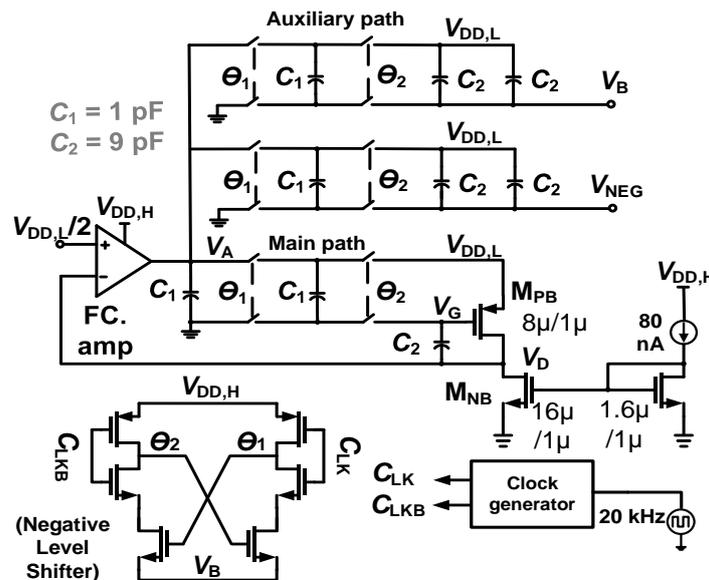
Figure 5. Schematic of negative voltage bias generator circuit.
