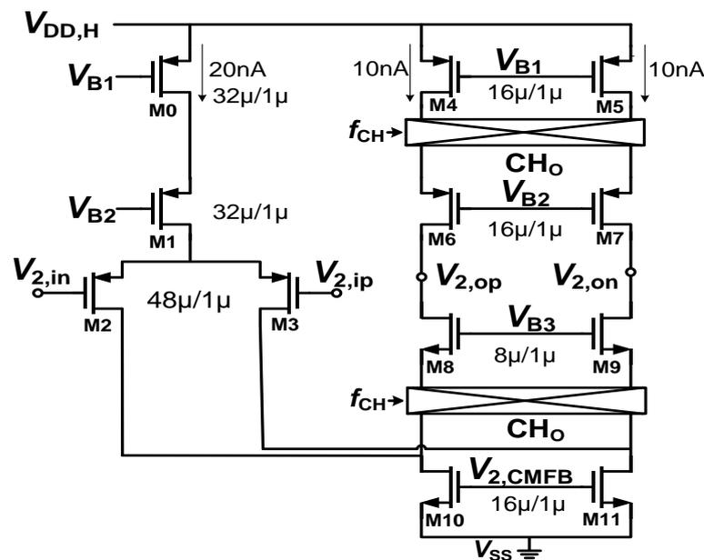
Figure 9. The schematic of the FC amp circuit.
