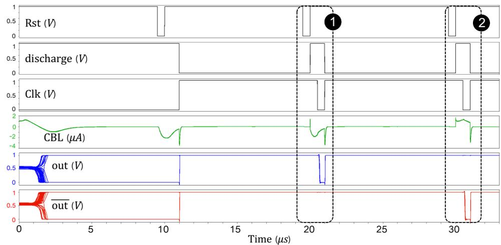
Figure 4. Transient simulation waveform of an 8 × 1 TCP array.
