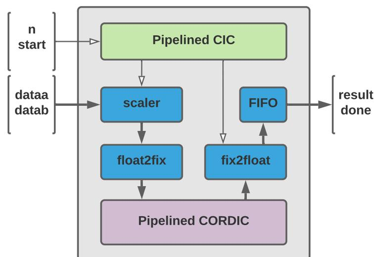
Figure 4. CORDIC Custom Instruction Basic Block Diagram.
