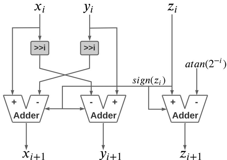
Figure 3. CORDIC calculation block.
