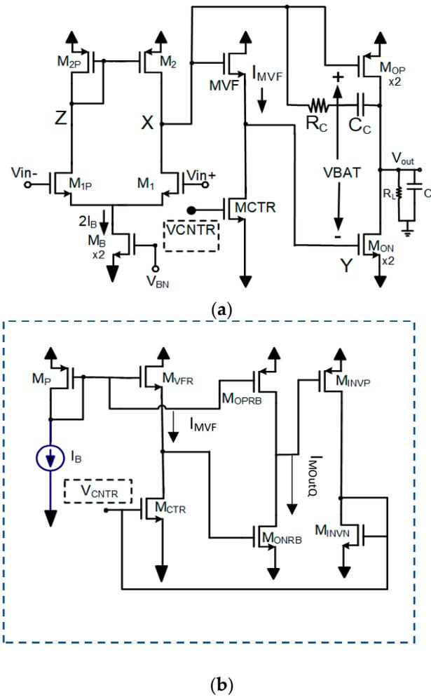
**Figure 2.** (a) Example of the class-AB output stage based on the floating battery principle using a VF with level shift and (b) a replica bias control circuit for the generation of VCNTR so that the quiescent output current has a nominal well-defined value independent of VDD, technology parameters, and temperature.
