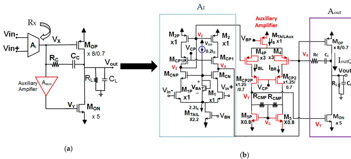
Figure 3. (a) Scheme of the proposed class-AB Miller op-amp and (b) transistor level implementation.
