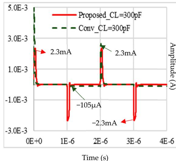
Figure 8. Current in the load capacitance  $C_L = 300\text{ pF}$  in the Conv-A and proposed op-amps for 500 kHz and 500 mV<sub>pp</sub> amplitude pulse inputs.
