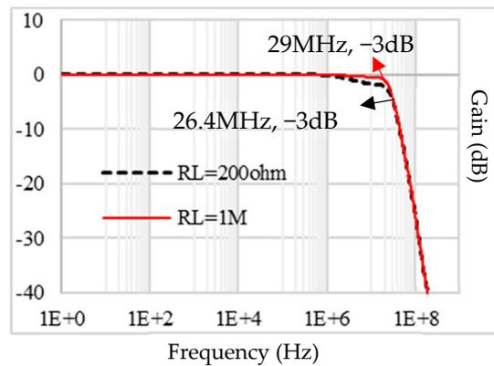
**Figure 11.** Frequency response of the proposed op-amp in a close-loop VF configuration for  $R_L = 1\text{ M}\Omega$  and  $R_L = 200\ \Omega$ .
