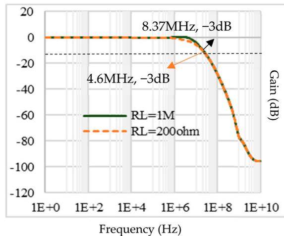
**Figure 12.** Closed-loop frequency response of the conventional class-A op-amp for  $R_L = 1\text{ M}\Omega$  and  $R_L = 200\ \Omega$  in the VF mode.
