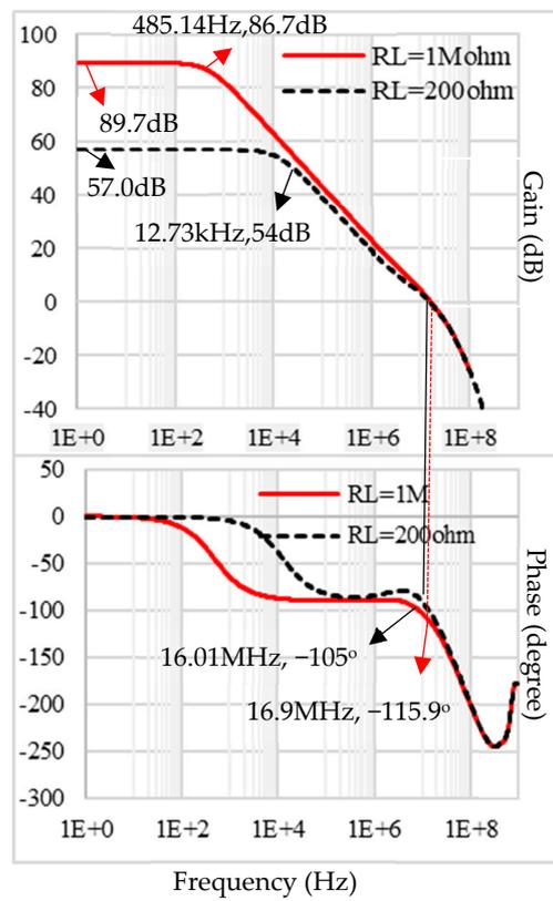
Figure 5. Frequency response of the proposed op-amp in open-loop configuration for  $R_L = 1\text{ M}\Omega$  and  $R_L = 200\ \Omega$ .
