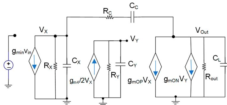
Figure 4. Small-signal model of the proposed op-amp.
