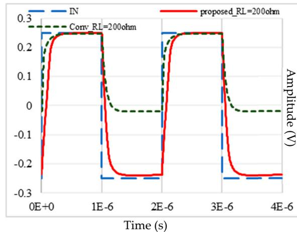
**Figure 9.** Transient response of the Conv-A and proposed op-amps for 500 kHz and 500 mV<sub>pp</sub> pulse inputs with  $R_L = 200 \Omega$  and  $C_L = 300 \text{ pF}$ .
