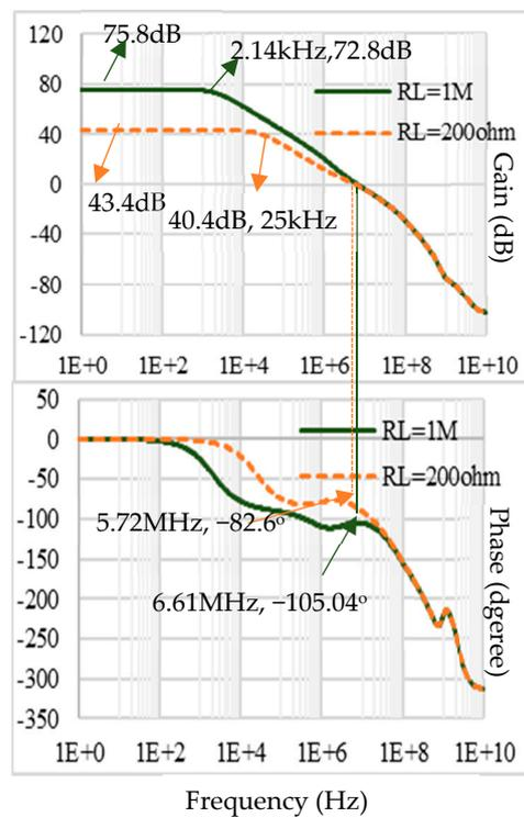
Figure 6. Open-loop frequency response of the Conv-A op-amp for  $R_L = 1\text{ M}\Omega$  and  $R_L = 200\ \Omega$ .
