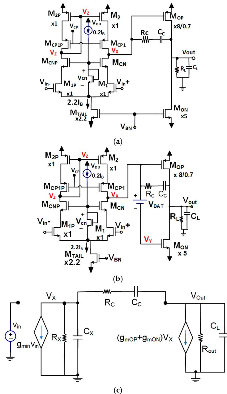
**Figure 1.** (a) Conventional class-A Miller op-amp, (b) Miller op-amp with class-AB output stage based on floating battery, and (c) small-signal model of the class-AB op-amp based on the floating battery scheme.
