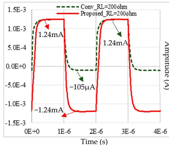
**Figure 10.** Current in  $R_L = 200 \Omega$  in the Conv-A and Proposed op-amps 500 kHz and 500 mV<sub>pp</sub> amplitude pulse inputs.
