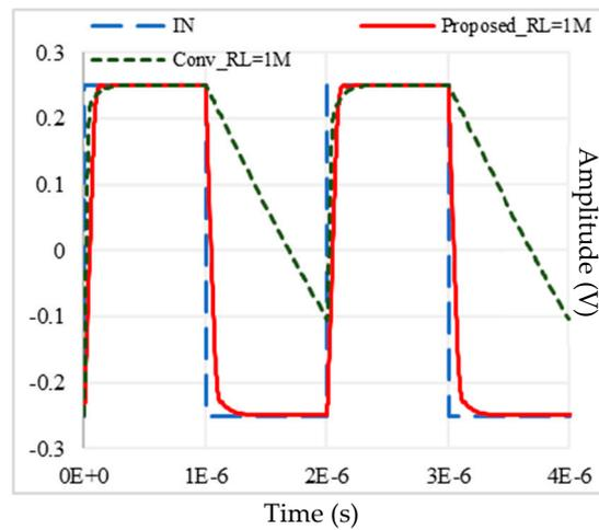
Figure 7. Transient response of the Conv-A and proposed op-amps for 500 kHz and 500 mV<sub>pp</sub> amplitude input pulses with  $R_L = 1\text{ M}\Omega$  and  $C_L = 300\text{ pF}$ .
