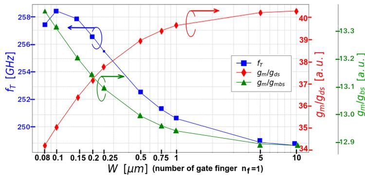
**Figure 2.** Obtained simulations for  $L = L_{min} = 30$  nm, indicated bias values and  $W$  sizes (finger = 1 for all cases). Please, observe that  $L$  is constant for all cases, hence, it is not necessary to plot  $W/L$  on the  $x$ -axis.
