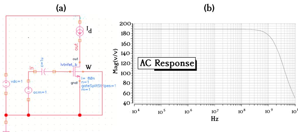
**Figure 5.** Case study: (a) common-source amplifier ( $L = 80$  nm). The  $I_d$  bias values and  $W$  sizes as indicated in Table 1, (b) simulated intrinsic-gain for the design case 1 (AC response). The theoretical intrinsic-gain is equal to  $g_m/g_{ds}$ .
