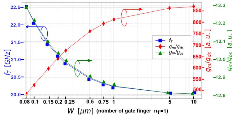
**Figure 3.** Obtained simulated for  $L = 180$  nm, indicated bias values and  $W$  sizes (finger = 1 for all cases). Please, observe that  $L$  is constant for all cases, hence, it is not necessary to plot  $W/L$  on the  $x$ -axis.
