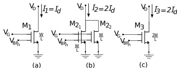
**Figure 1.** Scheme of compound UTBB FD-SOI transistors biased at the same  $g_m/I_d$  value, where  $V_G$  represents the gate voltage,  $V_D$  is the drain voltage and  $V_{BPn}$  is the back-gate bias voltage,  $I_1$ ,  $I_2$ ,  $I_3$  represent the drain bias current for each considered case, and  $W$  and  $L$  represent the width and channel length, respectively.
