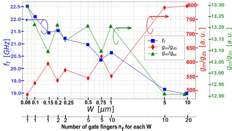
**Figure 4.** Obtained simulated parameters for  $L = 180$  nm, the indicated bias values and  $W$  sizes with indicated finger values. Please, observe that  $L$  is constant for all cases, hence, it is not necessary to plot  $W/L$  on the  $x$ -axis.
