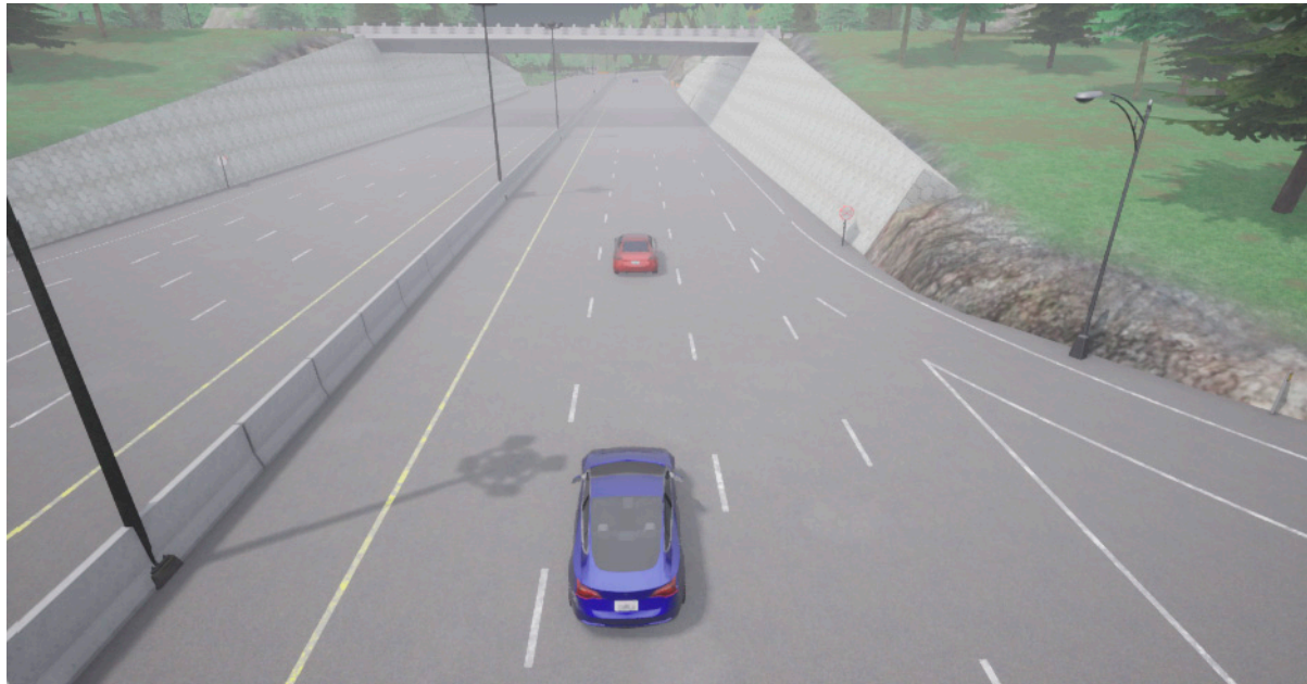
Figure 9. Example visualization of the simulation scenario in the CARLA environment during MRM execution. The red vehicle represents the ego vehicle, while the blue vehicles represent surrounding traffic participants.
