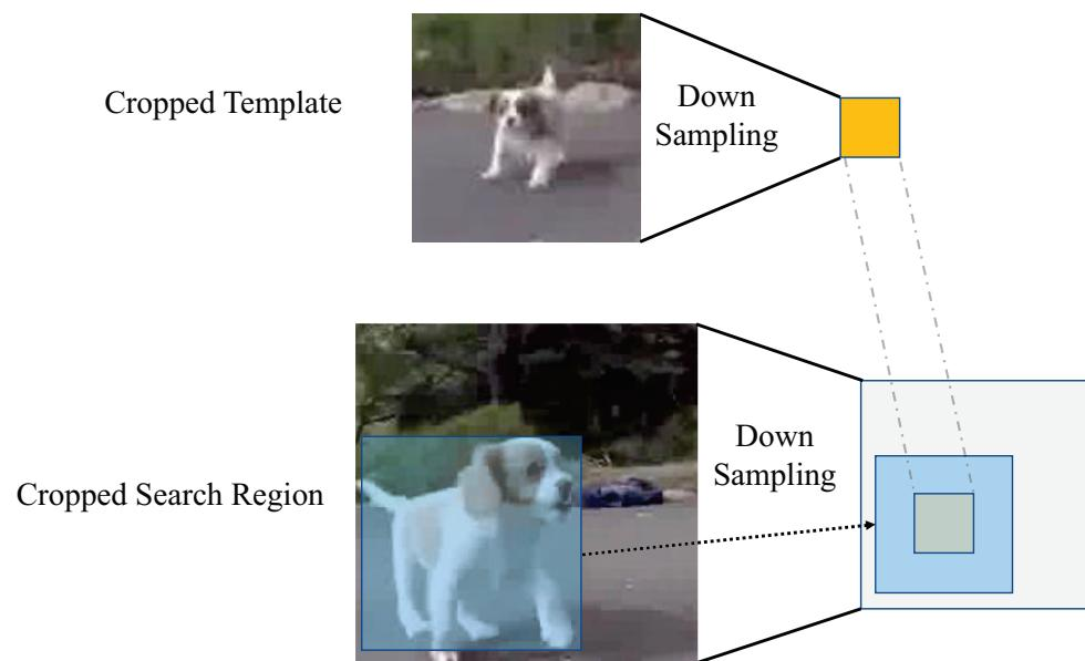
**Figure 4.** The effect of increasing the target's scale on Siamese networks.
