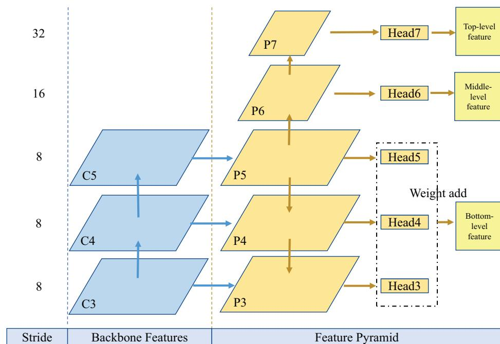
**Figure 7.** Architecture of multi-scale feature fusion network.
