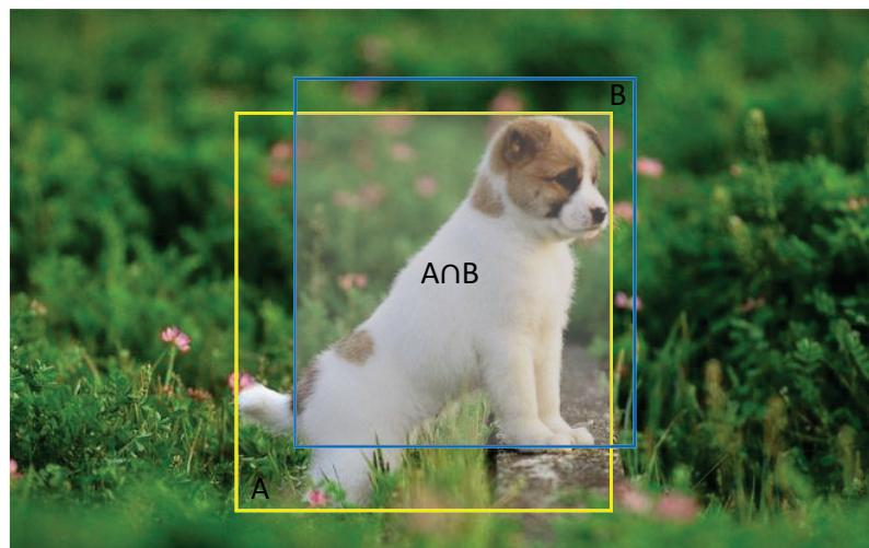
**Figure 14.** Example of IoU calculation method, where A represents the ground truth bounding box of the target and B represents the bounding box predicted by the algorithm.
