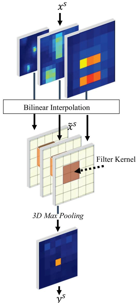
**Figure 9.** Schematic diagram of the process of 3D Max Filtering.
