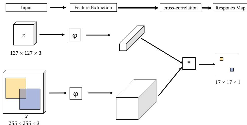
**Figure 1.** The network framework of SiamFC, where  $*$  represents the cross-correlation operation.
