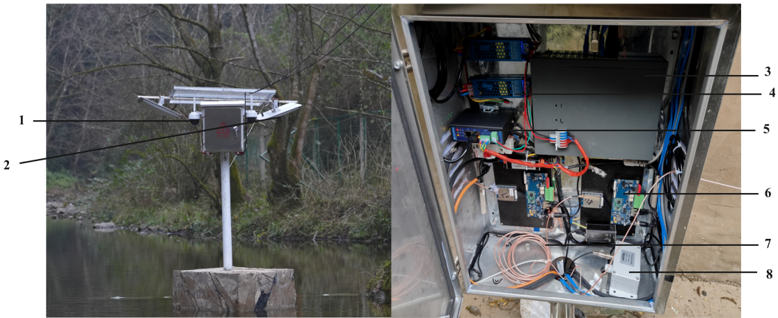
Figure 3. Schematic diagram of image acquisition device. 1. Camera for image capture. 2. Antenna for positioning. 3. Switch device. 4. Power supply unit. 5. Gateway interface. 6. Motherboard for positioning module. 7. Extension cable for positioning antenna. 8. Environmental sensor.
