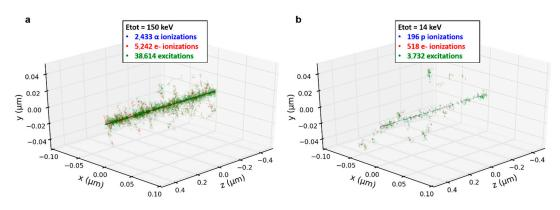
**Figure 4.** Track structures and number of ionizations of a single 3 MeV  $\alpha$ -particle and proton in water obtained with Geant4-DNA. The particles propagate along the *Z*-axis. When (**a**) one  $\alpha$ -particle and (**b**) one proton traverse 1  $\mu$ m of liquid water, the density of ionizations and the deposited energy (Etot) is about ten times higher for  $\alpha$ -particles than for protons, due to the  $\alpha$ -particle's higher LET.
