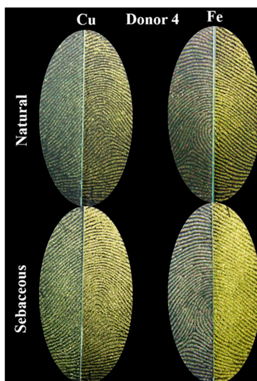
Figure 9. Half-and-half fingerprint (natural (N) and sebaceous (S)) from donor 4, with the left half developed using composites and the right half developed with Gold ® commercial powder purchased from Sirchie ® .
