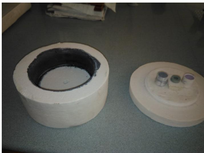
**Figure 1.** Capsule for a microwave kiln painted with SiC.
