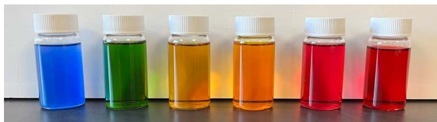
Figure 2. Final bulk dye solutions. From left to right: Phycobilin, Chlorophyll, \alpha -Mangostin, Curcuminoids, Anthocyanin, Betalin. Note that while the extracts are purported to be single-chemical species in Table 1, they are actually combinations of multiple substituted variants of the parent molecule of the dye class.
