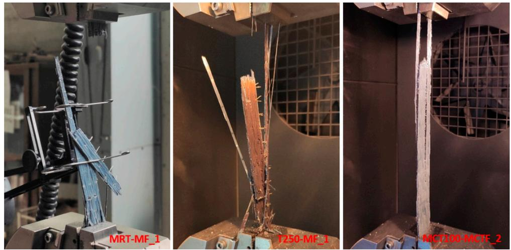
Figure 6. Mode of failure of the specimens.
