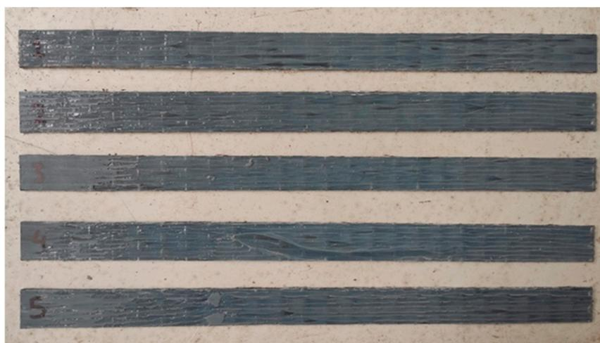
**Figure 1.** Investigated specimens (MRT-MF\_1;  $t = 1.63\text{ mm}$ ,  $b = 15.74\text{ mm}$ , MRT-MF\_2;  $t = 1.74\text{ mm}$ ,  $b = 17.26\text{ mm}$ , MRT-MF\_3;  $t = 1.71\text{ mm}$ ,  $b = 14.68\text{ mm}$ , MRT-MF\_4;  $t = 1.65\text{ mm}$ ,  $b = 16.56\text{ mm}$ , MRT-MF\_5;  $t = 1.78\text{ mm}$ ,  $b = 15.95\text{ mm}$ ).
