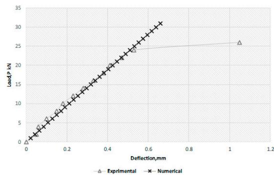
Figure 27. Load–deflection diagram of beam (B5).
