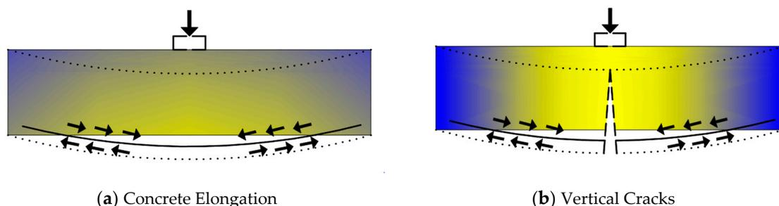
Figure 15. Cracks pattern at ultimate load.
