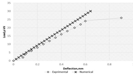
Figure 25. Load–deflection diagram of beam (B3).
