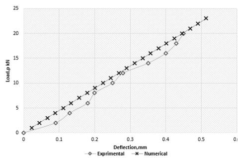
Figure 23. Load-deflection diagram of beam (B1).
