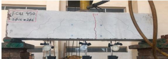
(b) Experimental crack pattern
