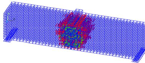
(c) Numerical crack pattern
