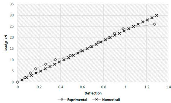
Figure 26. Load–deflection diagram of beam (B4).
