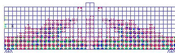
(c) Numerical crack pattern
