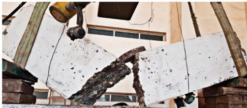
(b) Experimental crack pattern
