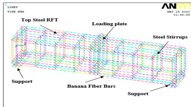
Figure 13. Model of reinforcement of beams (B2 to B5).
