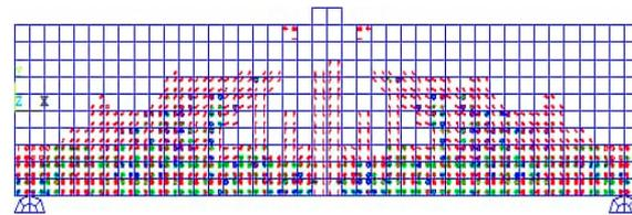
(c) Numerical crack pattern
