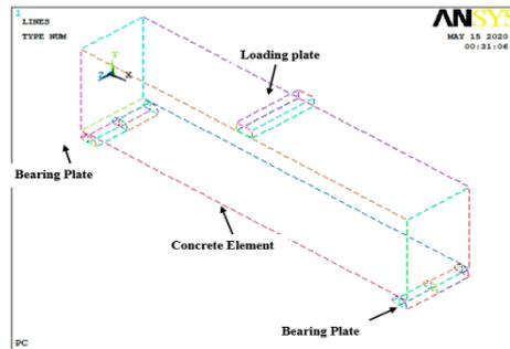
Figure 11. Modeling of beam (B1).
