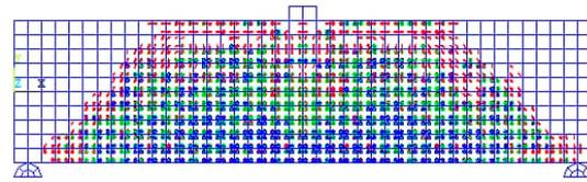
(c) Numerical crack pattern
