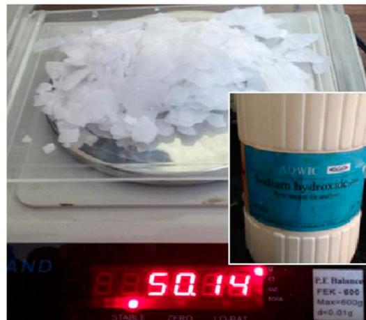
**Figure 2.** Sodium hydroxide alkali treatment.
