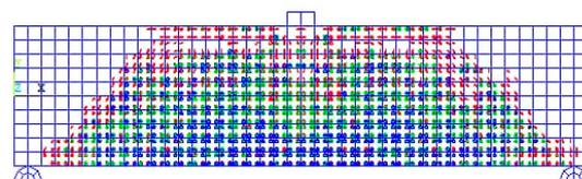
(c) Numerical crack pattern
