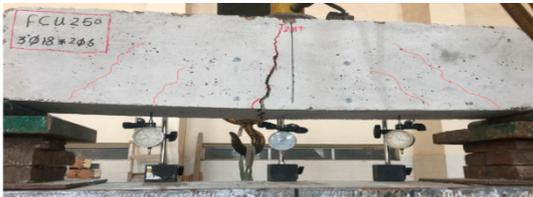
(b) Experimental crack pattern
