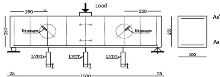
Figure 12. Details of the tested beams and instrumentations.
