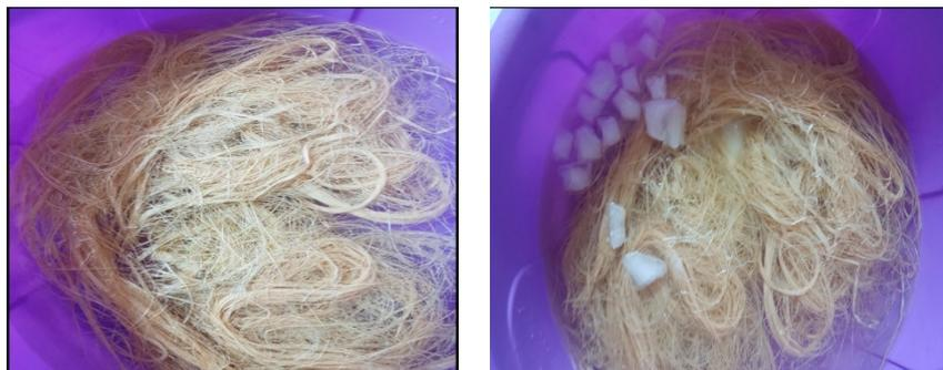
**Figure 3.** Submerging banana fibers in NaOH solution.
