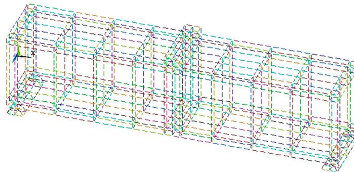
Figure 8. Typical idealization of the steel stirrups, top, and bottom bars.
