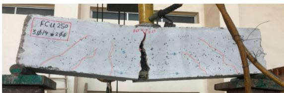
(b) Experimental crack pattern
