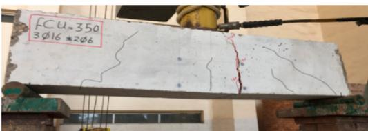
(b) Experimental crack pattern
