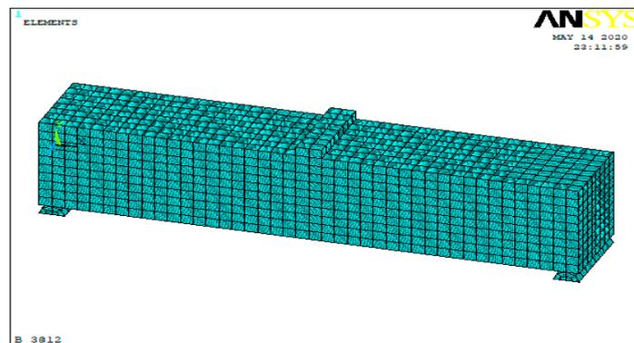
**Figure 7.** Typical idealization of the beam element.
