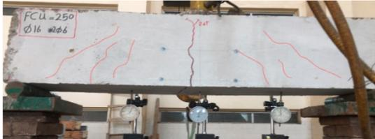
(b) Experimental crack pattern
