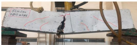
(b) Experimental crack pattern
