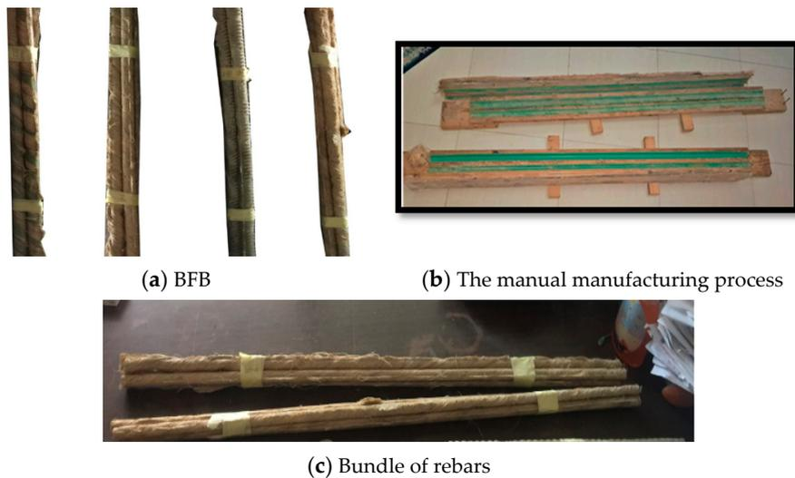
**Figure 4.** Shapes and manufacturing process of banana fiber bars.
