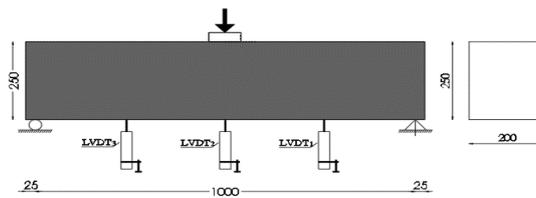
Figure 10. Details of the tested beam (B1).
