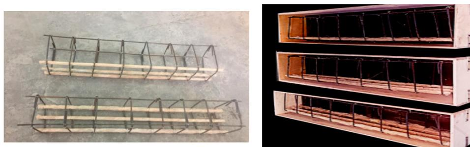
**Figure 5.** BFRP bars as reinforcement of the tested beams.
