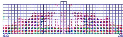
(c) Numerical crack pattern
