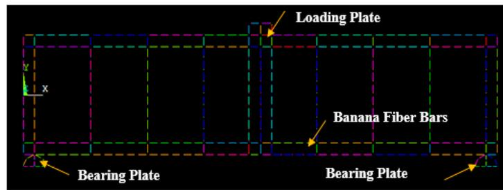
Figure 14. Reinforcement modeling for beams (B4, B6, and B7).
