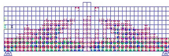
(c) Numerical crack pattern
