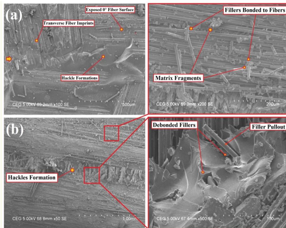
**Figure 11.** Fractured surfaces of (a) baseline glass/epoxy samples (b) 5% wt. filler modified glass/epoxy samples. To the right, two insets of (b) showing close-up of the marked regions.
