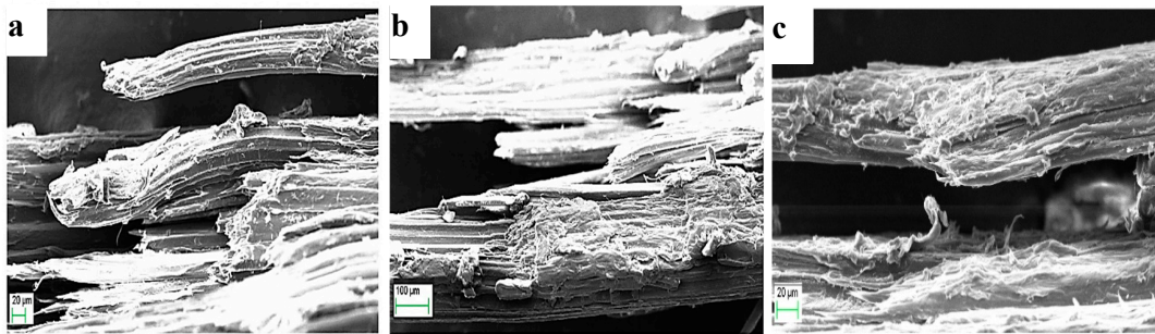
Figure 2. Microstructure of the surface of 2 wt.% NaOH-treated concentration the single-cellulosic Buluh semantan strips after soaking for 12 h in 2 wt.% NaOH showing in (a–c) fractured fibers in different magnification.
