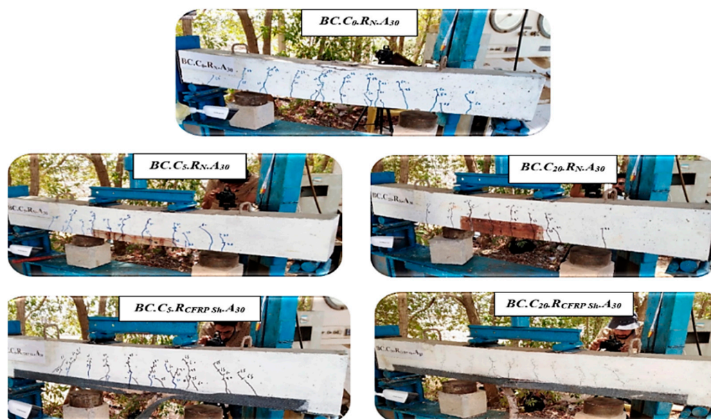
Figure 7. Cracking patterns at failure for specimens in group B.
