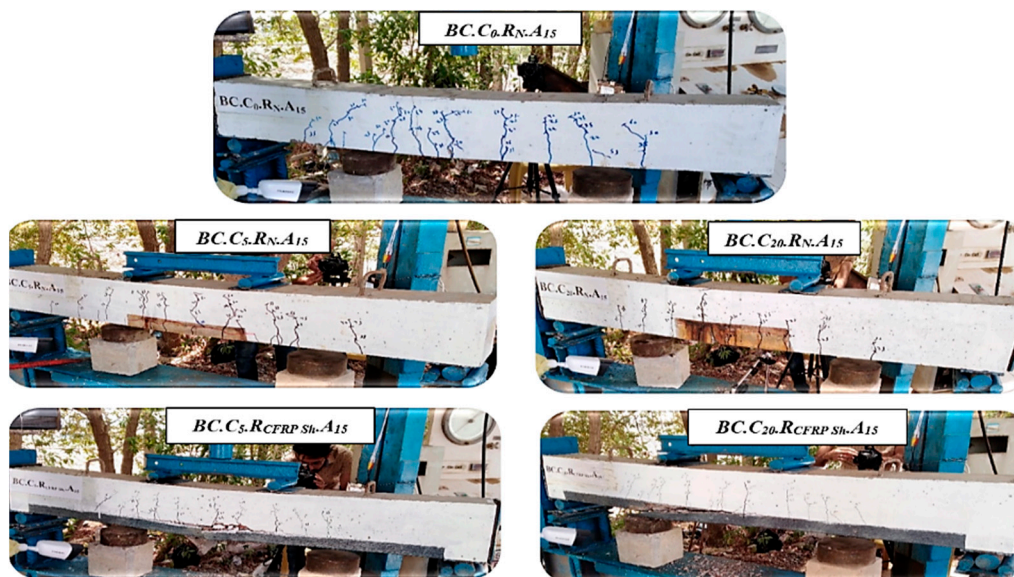
Figure 6. Cracks pattern at failure for specimens in group A.
