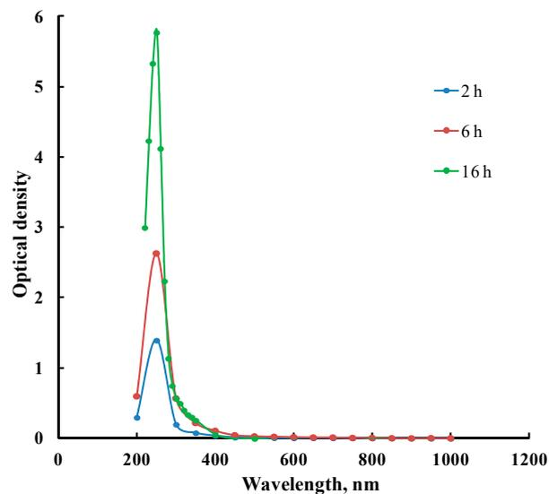
**Figure 2.** The polyethylene glycol (PEG) optical spectra after the thermal treatment at 120 °C with respect to the initial PEG.
