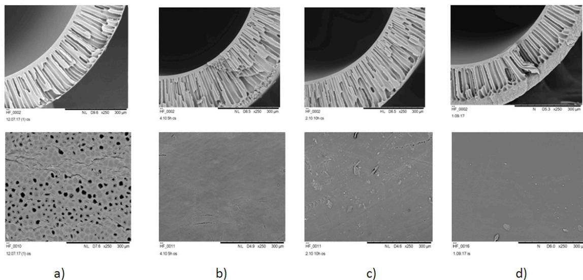
**Figure 7.** SEM images of the cross-sections (upper row) and the outer surface (lower row) of the hollow fiber membranes obtained from solutions with different time of thermal treatment at 120 °C: (a) 6 h, (b) 11 h, (c) 16 h, (d) 24 h.
