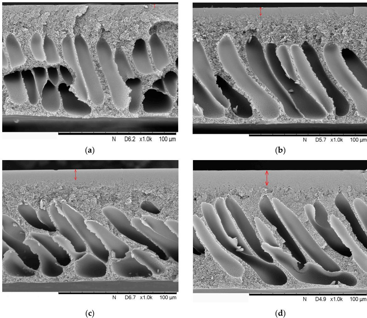
**Figure 6.** Scanning electron microscopy (SEM) micrographs of flat PSf membranes obtained from solutions with different time of thermal treatment at 120 °C (a) 6 h, (b) 11 h, (c) 16 h, (d) 24 h.
