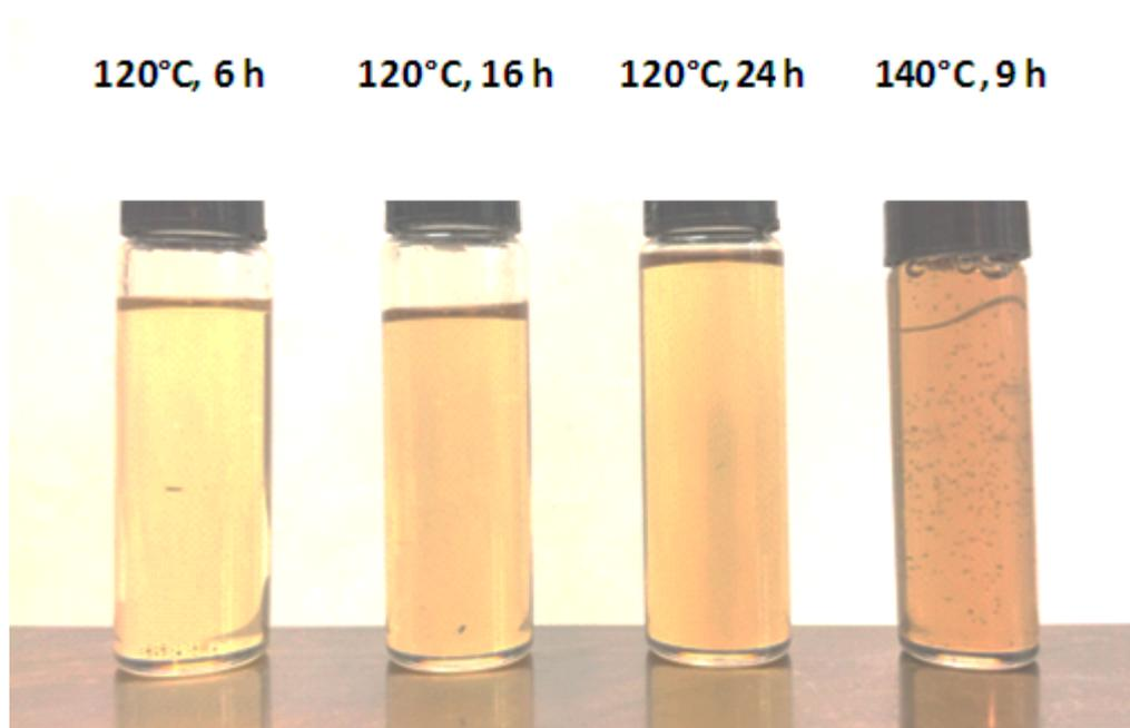
**Figure 1.** Photographs of casting solutions obtained at different times and temperatures of mixing.
