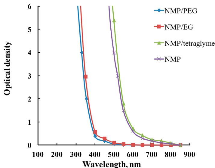
**Figure 4.** The optical spectra of NMP, NMP/PEG, NMP/ethylene glycol (EG), and NMP/tetraglyme after the thermal treatment at 120 °C for 24 h with respect to the initial samples.
