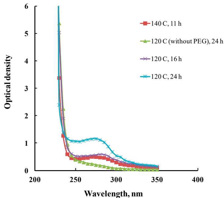
**Figure 5.** The optical spectra of the water phase after polysulfone (PSf) precipitation with respect to the water phase without PEG.
