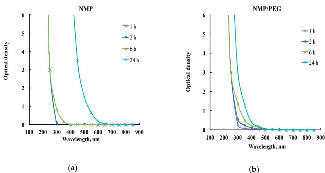
**Figure 3.** The N-methyl-2-pyrrolidone (NMP) and NMP/PEG (75/25) optical spectra after the thermal treatment at 120 °C with respect to the initial NMP (a) and NMP/PEG (b).
