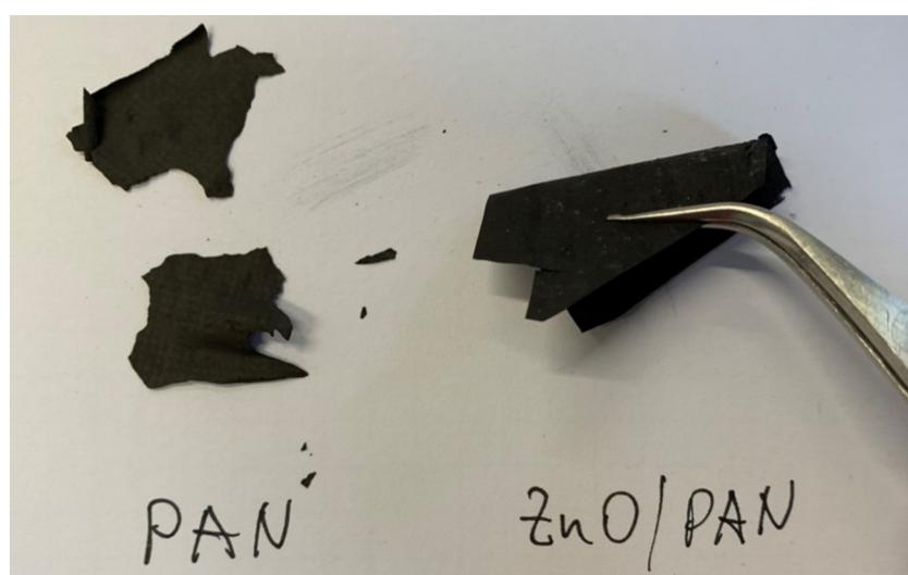
**Figure 5.** Bending a carbonized PAN nanofiber mat (stabilized without fixation) only slightly results in brittle failure (**left** side), while bending carbonized PAN/ZnO nanofiber mats (stabilized without fixation) is possible with a narrow bending radius (**right** side).
