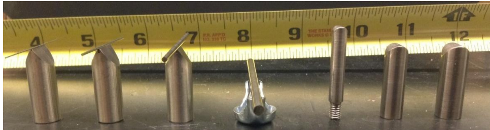
Figure 2. Seven different indenters used in transverse loading experiments. From left to right, the indenters possess radii of curvature of 0.20, 0.40, 0.79, 1.59, 2.50, 3.81, and 4.50 mm.
