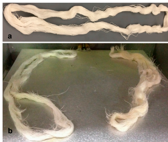
Figure 1. (a) Control cotton yarn with no plasma exposure and no visual yarn breakages and (b) the visual breakages observed after plasma degradation of yarns exposed to 90 min plasma exposure at 0.46 \text{ W/cm}^2 .
