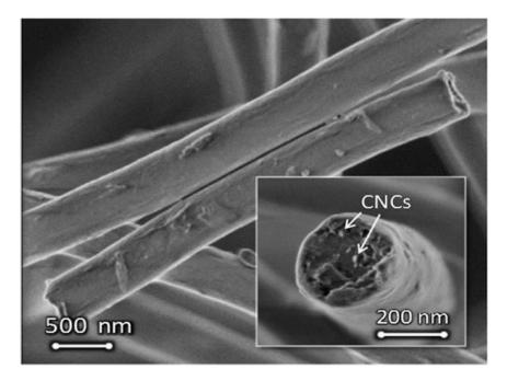
**Figure 13.** SEM images of lignin/polyvinyl alcohol (PVA)/cellulose nanocrytals (CNC) composite nanofiber, with an inset image of the cross-section of the said composite prepared by the freeze crack method [195]. Reproduced with permission from ref. [195]. Copyright American Chemical Society, 2012.
