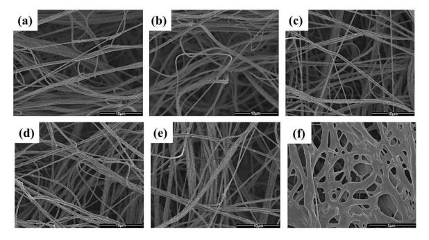
**Figure 18.** SEM images of solution blown chitosan/PVA nanofibers with different ethylene glycol diglycidyl ether (EGDE) content: (a) 7%; (b) 5%; (c) 4%; (d) 3%; (e) 2%; and (f) the swollen chitosan/PVA/EGDE-7% [253]. Reproduced with permission from ref. [253]. Copyright Elsevier, 2014.
