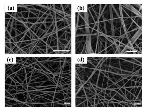
**Figure 10.** SEM images of electrospun chitosan fibers: (a) Low MW; (b) medium MW; (c) high MW; and (d) practical grade. The scale bars in all the images are 1  $\mu$ m, except in (d), where the scale bar indicates 500 nm. Reproduced with permission from ref. [160]. Copyright American Chemical Society, 2008.
