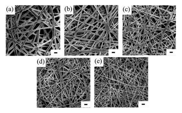
**Figure 15.** SEM images of soy protein isolate (SPI)/ polyamide 6 (PA6) nanofibrous membranes with different SPI/PA6 mass ratios: (a) 1:9; (b) 2:8; (c) 3:7; (d) 4:6; and (e) 5:5. Scale bar = 1  $\mu$ m [168]. Reproduced with permission from ref. [168]. Copyright John Wiley and Sons, 2017.
