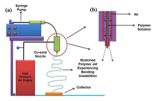
**Figure 3.** Schematic representation of solution blowing: (**a**) The overall view and (**b**) the zoomed in view of the solution blowing co-axial nozzle.
