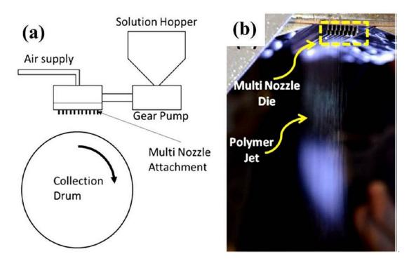
**Figure 17.** (a) Schematic of the industrial-scale solution blowing setup, as shown in Kolbasov et al., (2015); (b) actual multi-nozzle solution blowing process using BIAX die nosepiece. Reproduced with permission from ref. [47]. Copyright American Chemical Society, 2016.
