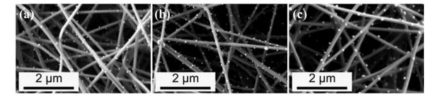
**Figure 14.** SEM images of Ag/cellulose nanofibers (CNFs) with the Ag loading amounts being (**a**) 11 wt. %; (**b**) 15 wt. %; and (**c**) 25 wt. % [190]. Reproduced with permission from ref. [190]. Copyright Elsevier, 2014.
