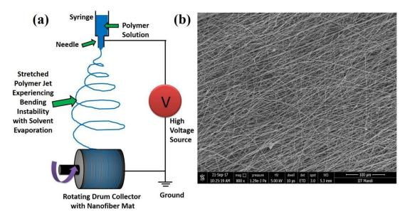
**Figure 2.** (**a**) Schematic representation of the Electrospinning process and (**b**) electrospun nonwoven mat of Polyacrylonitrile (PAN) from an unpublished work of authors.
