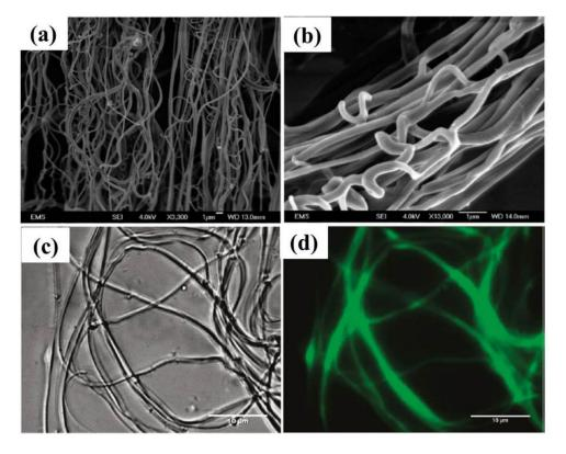
**Figure 16.** (**a**,**b**) SEM images of SPI/Nylon 6 blend monolithic fibers; (**c**,**d**) optical and fluorescent images of the same fibers, respectively, where the green color in image (**d**) proves the existence of SPI in fibers [248]. Reproduced with permission from ref. [248]. Copyright American Chemical Society, 2011.
