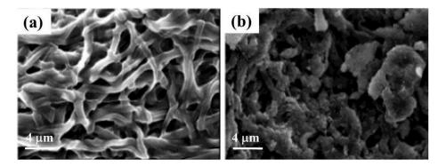
**Figure 7.** SEM images of oxidized cellulose acetate nanofibers (**a**) In HNO<sub>3</sub>/H<sub>3</sub>PO<sub>4</sub>-NaNO<sub>2</sub> solvent (**b**) in HNO<sub>3</sub>/H<sub>2</sub>SO<sub>4</sub>-NaNO<sub>2</sub> solvent shown [113]. Reproduced with permission from ref. [113]. Copyright American Chemical Society, 2004.
