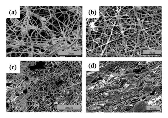
**Figure 12.** SEM images of (**a**) 1.5 L; (**b**) 2.0 L; (**c**) 2.5 L; and (**d**) 3.0 L electrospun nanofibers [197]. Reproduced with permission from ref. [197]. Copyright Springer Nature, 2014.
