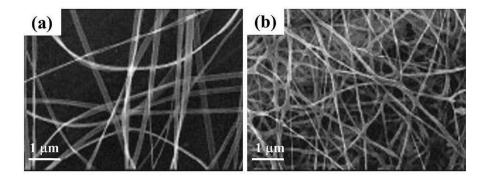
**Figure 6.** Shows cellulose acetate nanofibers in acetone/H<sub>2</sub>O solvent. (**a**) Normal cellulose nanofibers (**b**) deacetylated after 1 min [96]. Reproduced with permission from ref. [96]. Copyright John Wiley and Sons, 2013.
