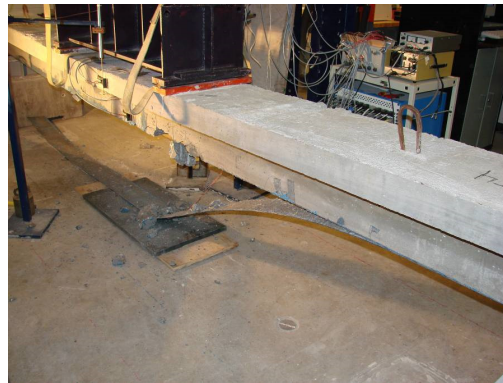
Figure 5. Beam T2 at failure.
