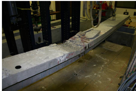
Figure 3. Beam T1 at failure.
