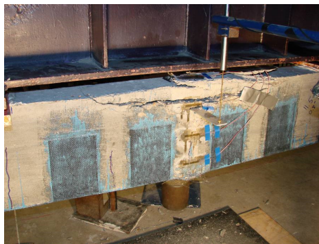
Figure 13. Beam R3 at failure.
