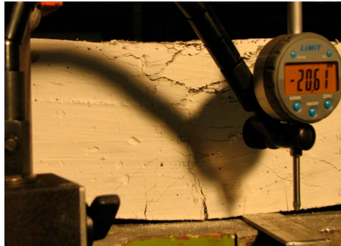
Figure 10. Reinforced concrete beam specimen with polypropylene fiber at failure.
