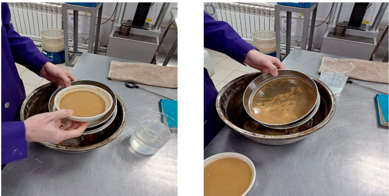
Figure 4. Determination of porosity and particle separation of the processed basalt insulation waste.
