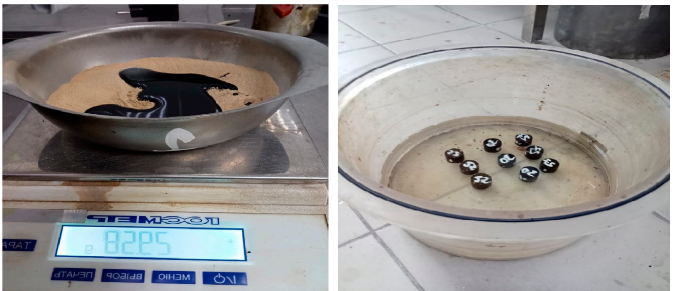
Figure 6. Swelling of samples from the mixture of powder with bitumen.
