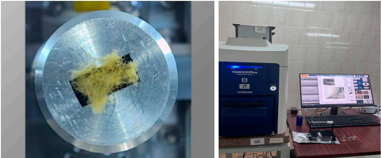
Figure 3. Chemical composition determination by X-ray spectroscopy (EDS).
