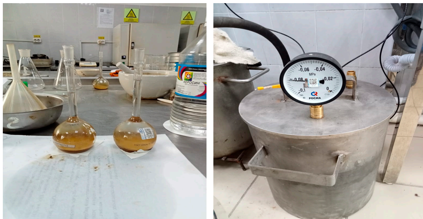
Figure 8. Determination of the moisture content of the mineral powder.
