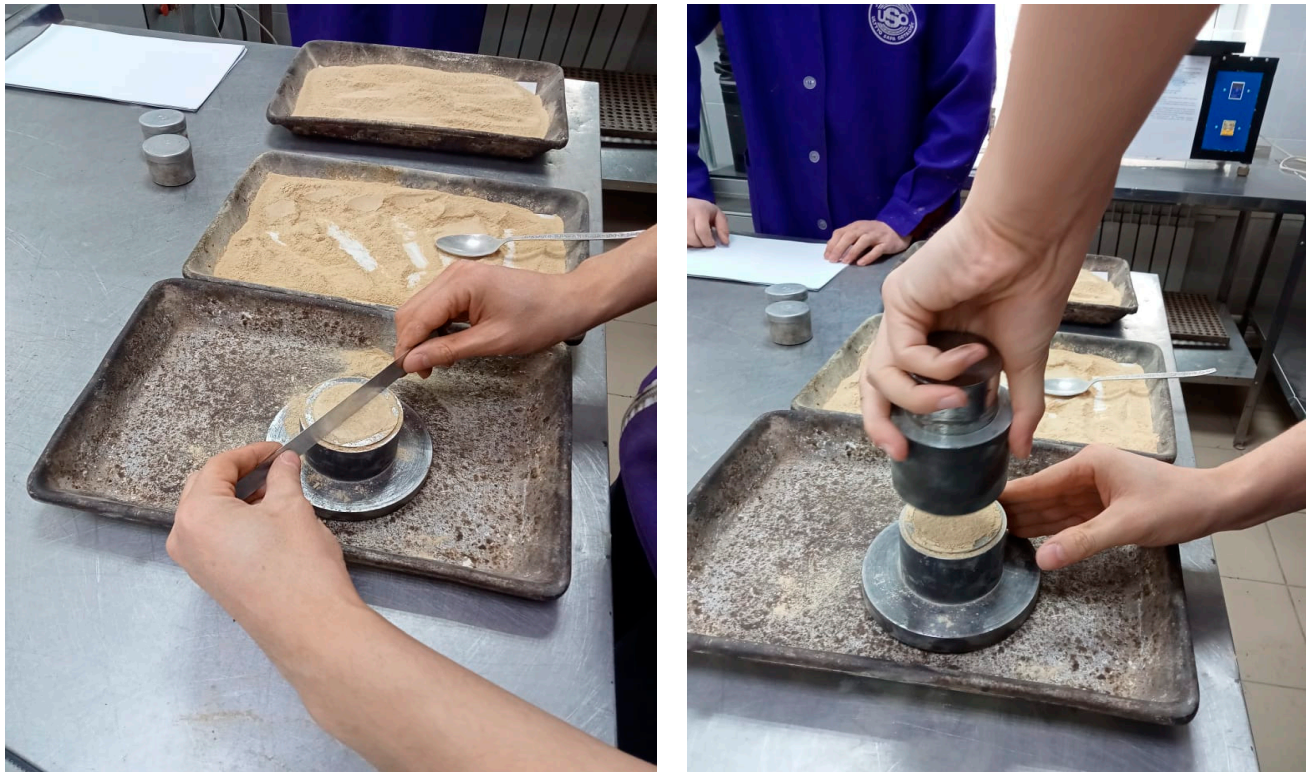
Figure 5. Determination of the true density of mineral insulation waste particles using a volumetric compaction device.
