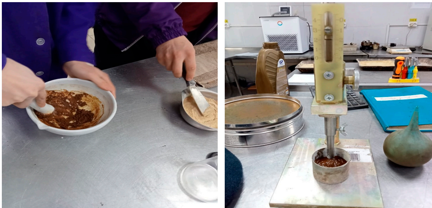
Figure 7. Manual mixing of the mineral powder with bitumen, and subsequent determination of its bitumen capacity using a standardized plunger device.
