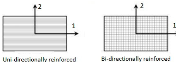
Figure 3. Examples of sheets with orthotropic material directions (1, 2).
