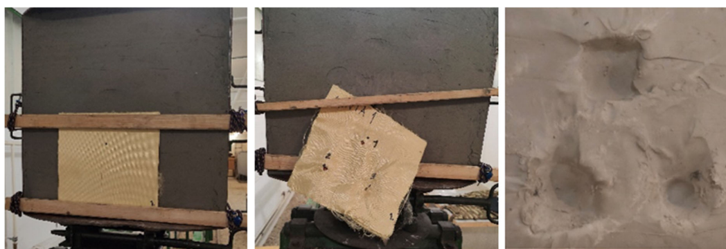
Figure 8. The neat Kevlar specimen before and after the shots, and the trauma zone.
