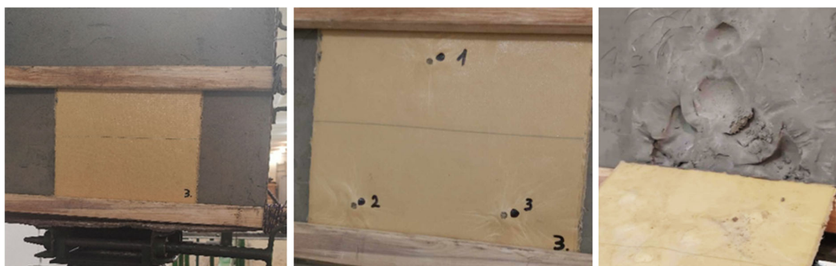
Figure 10. The Polyurethane/Kevlar specimen before and after the shots, and the trauma zone.
