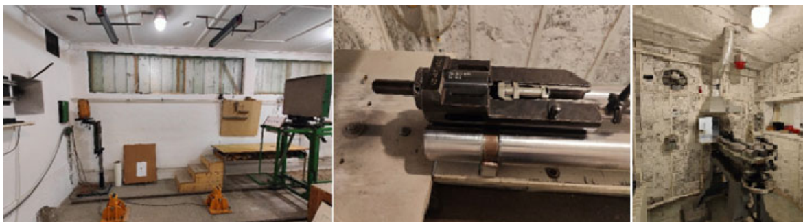
Figure 4. Experimental setup in the ballistics laboratory from left to right: infrared gates for measuring projectile velocity, gun barrel for firing 9 mm projectiles, gun stand.
