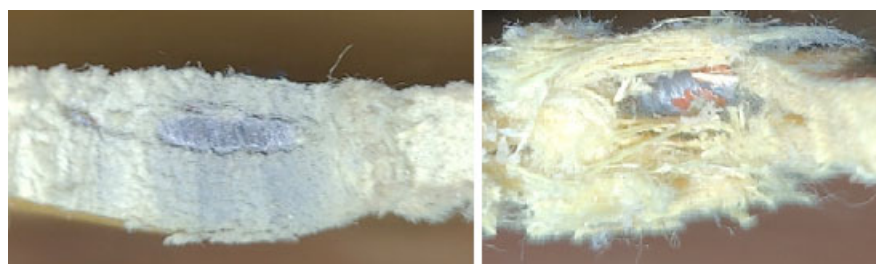
Figure 12. Cross-sectional images of projectiles fired into Epoxy/Kevlar ( left ) and into Polyurethane/Kevlar ( right ) specimens.
