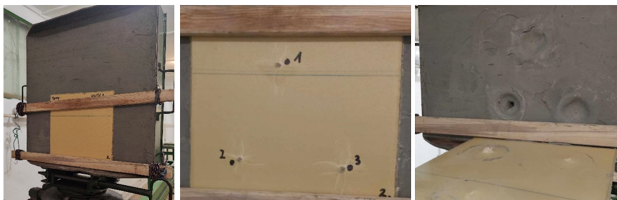
Figure 9. The Epoxy/Kevlar specimen before and after the shots, and the trauma zone.
