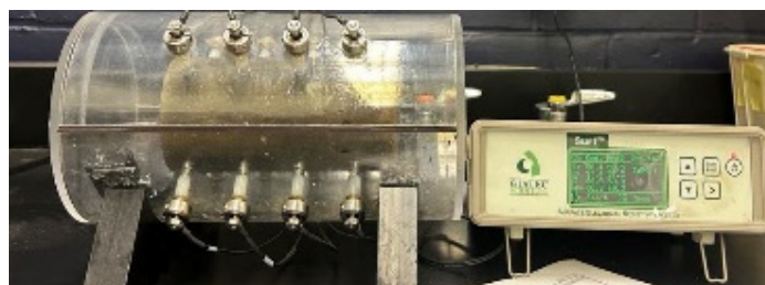
Figure 1. Electrical surface resistivity testing on 3'' \times 6'' cylinders.
