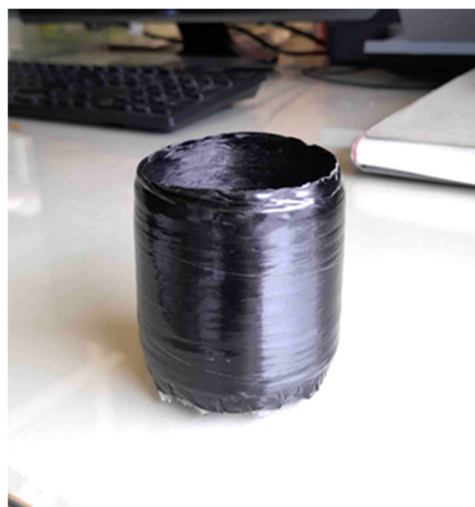
Figure 1. Custom-manufactured CFRP composite cylinder produced via filament winding.
